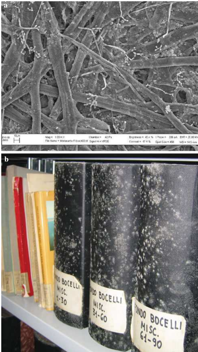
Fig. 9.7 (a) Scanning Electron Microscope (SEM) image. Paper attacked by a cellulolytic species of Cladosporium . SEM ZEISS EVO50, High Vacuum, observation of a non-metallised sample. (b) Books on metal shelving; their covers have been damaged by mould
