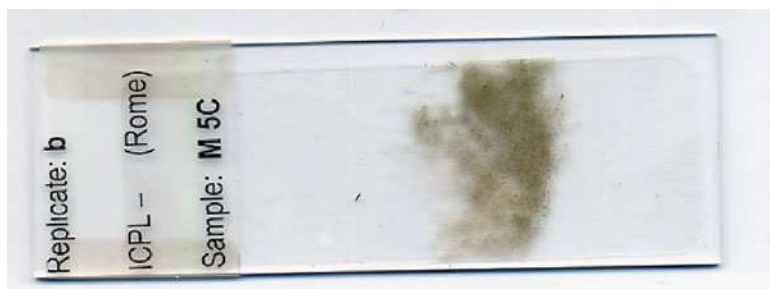
Fig. 11.6 A fragment of adhesive tape used for sampling the mould efflorescence present on volumes in the Angelica Library. The mould appeared whitish in colour when observed on materials and green-dull grey when sampled using transparent tape
