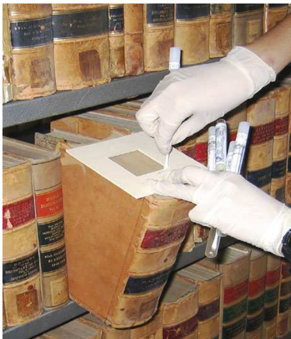
Fig. 9.10 Standardised swab sampling of dust from books’ surface using a 5×5 cm frame
