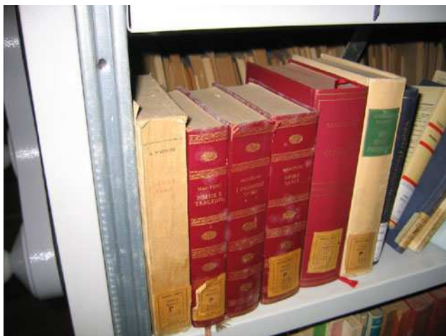
Fig. 11.2 Volumes stored in compactus-type shelving units and affected by moulds at the Estense Public Library. Only books with bindings made of leather, parchment or canvas presented with mould growth
