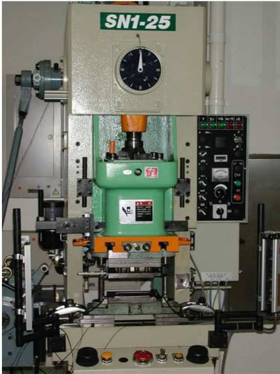
Fig. 1.4 A typical stamping machine (BowStar Biz Management Ltd)
