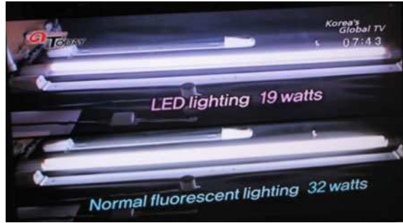
Fig. 5.5 LED lighting and normal fluorescent lighting illumination
