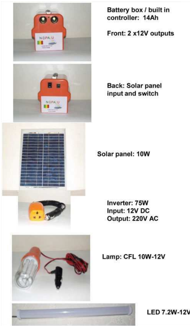
Fig. 2.37 Individual elements of the lighting photovoltaic kit
