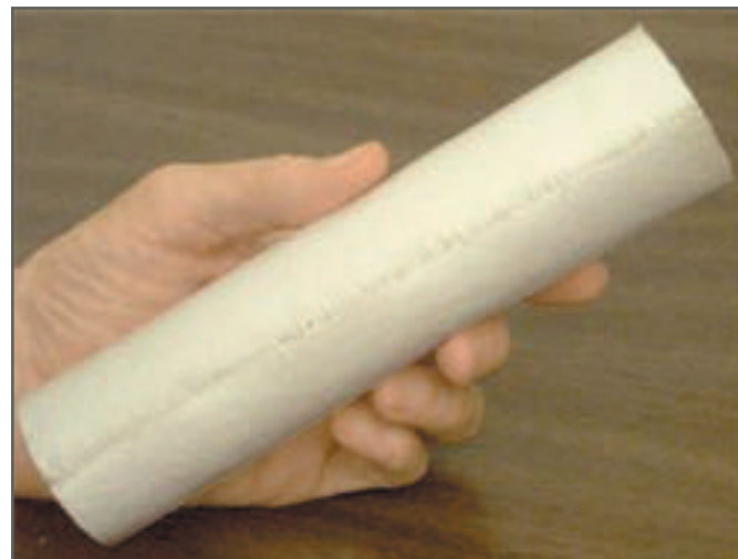
Separator tube after bonding
