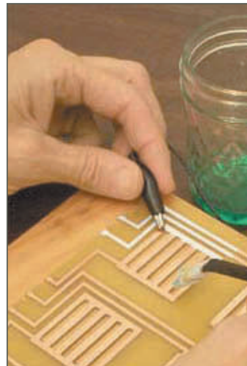
Applying nickel plating over the copper layer
