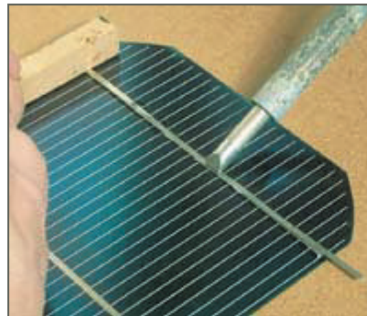
Soldering tab ribbon to the cell front (above) and cell back (below).
