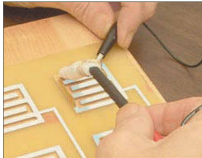
Applying gold plating over nickel plating
