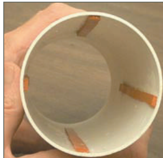
Glue rubber spacers on the inside of the electrolyzer tube
