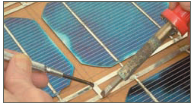
Connect the strings with small pieces of bus wire.
