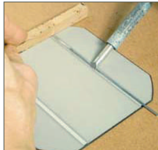
Soldering tab ribbon to the cell front (above) and cell back (below).
