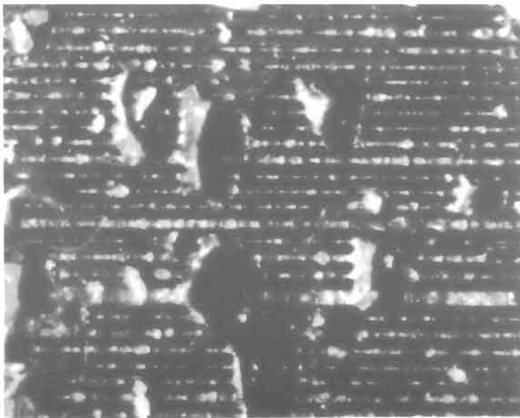
Fig. 36.11. Photomicrograph of fracture face showing primary failure mode interfacial failure between the boron fibers and the epoxy matrix.
