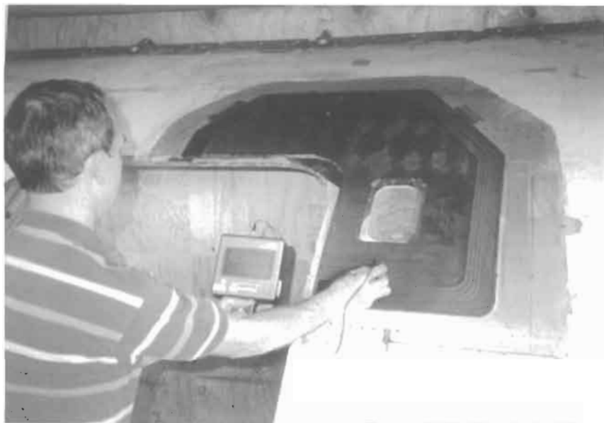
Fig. 23.4. Pulse-echo ultrasonic inspection of door corner composite doubler using a Quantum A-scan device.
