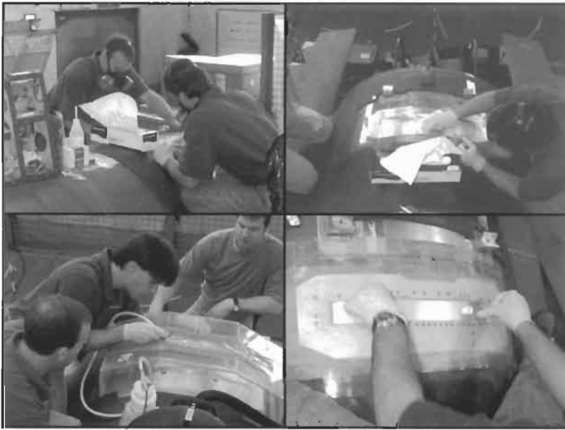
Fig. 26.1. ARTI technicians in a typical hangar environment performing (a) solvent scrub, (b) water wipe, (c) grit blast and (d) laminate application for repair of an F-16 FS 479 bulkhead.
