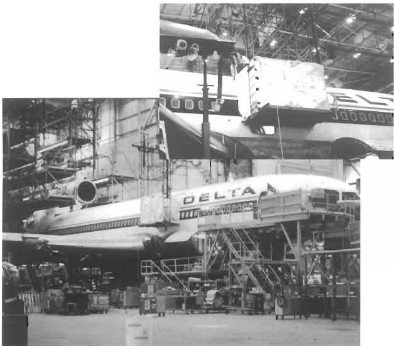
Fig. 28.13. Delta L-1011 aircraft during installation of composite doubler (inset – work stand positioned next to the right side passenger door).
