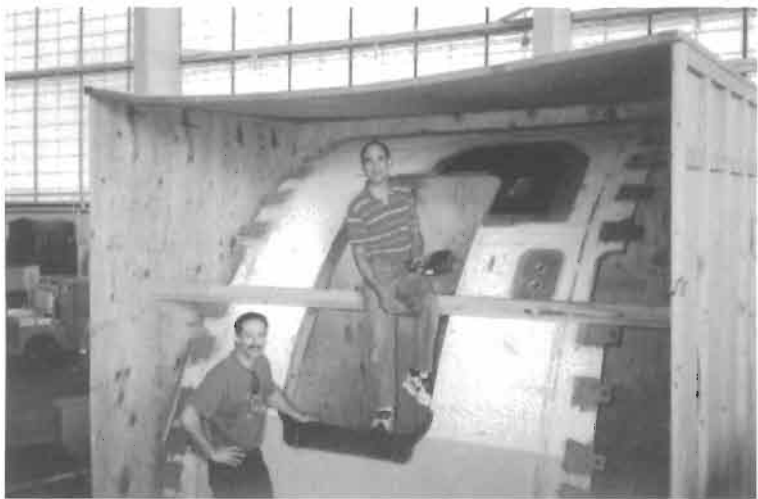
A. Fuselage Test Article with Composite Doubler Installed; Note Reinforcing Plates Around Perimeter of Fuselage Section for Load Application
