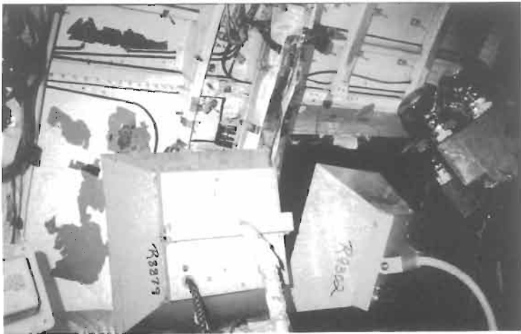
Fig. 28.18. Heat lamps positioned inside aircraft to help maintain cure temperature on back skin.
