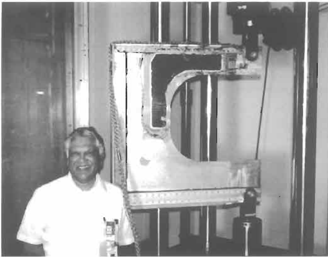
Fig. 28.9. Photograph of door corner test article mounted in a uniaxial test machine.
