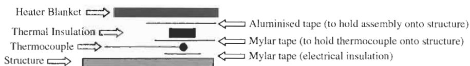
Fig. 24.11. Method for installation of thermocouples for measuring surface temperatures.
