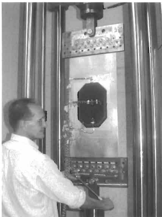
Fig. 35.7. Set-up for DC-10 composite doubler validation test.
