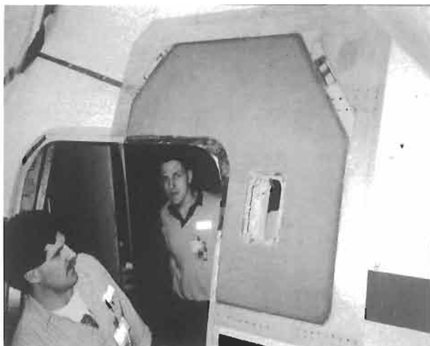
Fig. 28.19. Composite doubler following cure process (prior to application of delta paint scheme).
