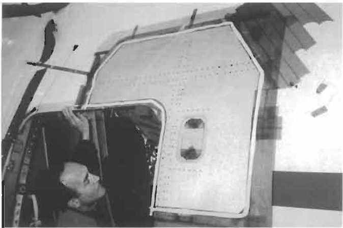
Fig. 28.14. Anodized door corner prepared for doubler bonding process.
