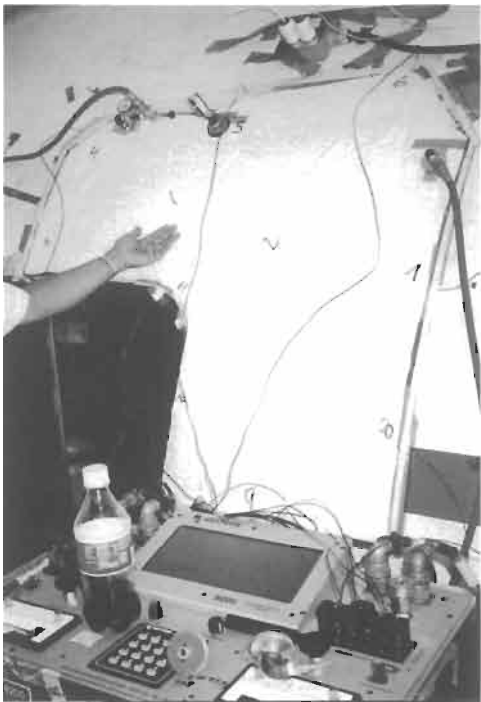
Fig. 28.17. Cure process – doubler beneath heat blanket, insulation, and vacuum bag assembly; heat controller is shown in foreground.
