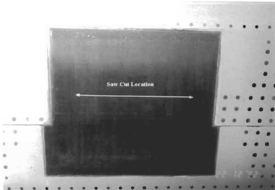
Fig. 16.24. Doubler installed on A330 lap joint.
