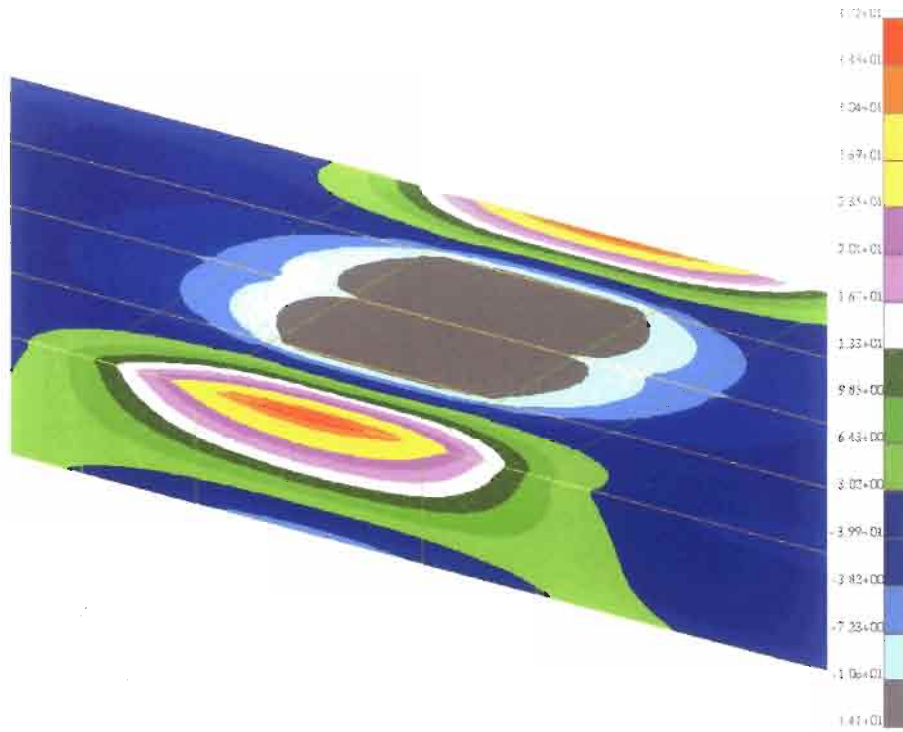
Fig. 11.20. Spanwise stresses corresponding to thermal loading as a result of heating. (This model does not include the patch). Note the tension stresses on the top edge of the wing.
