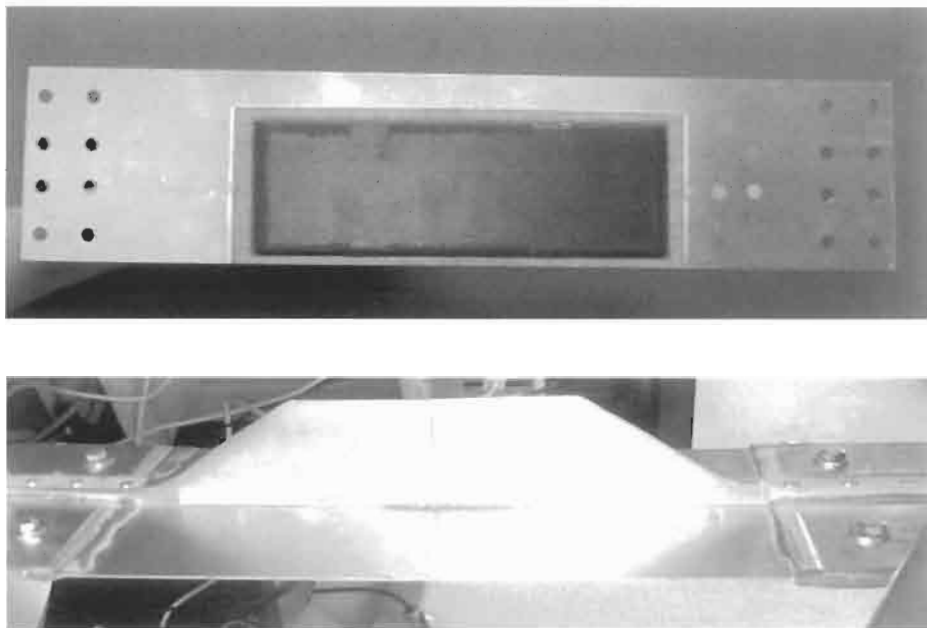
Fig. 9.6. View of patched surface and underside of the test configuration with cracked stiffener. Note adhesive seepage through the rivets.
