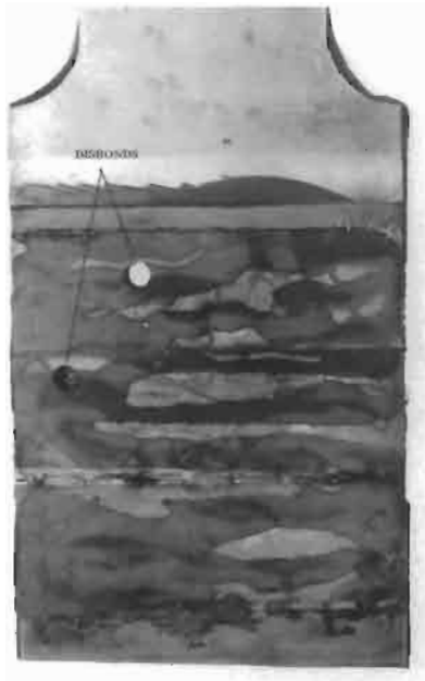
Fig. 16.19. Specimen A10 with doubler removed.
