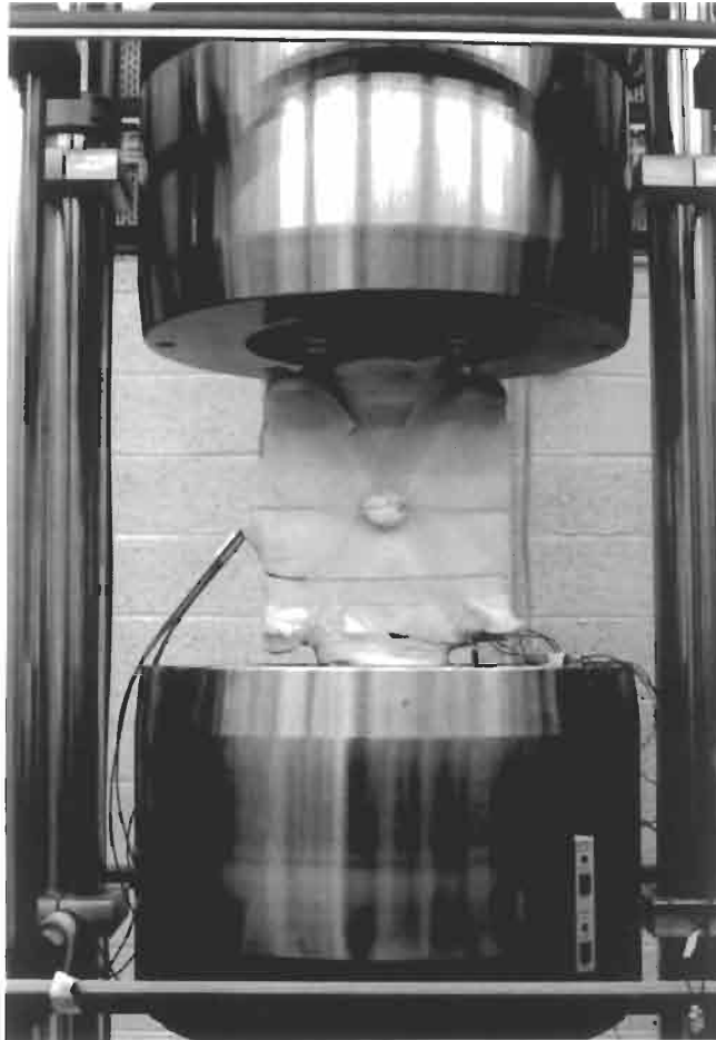
Fig. 16.18. Environmental fatigue test set-up.
