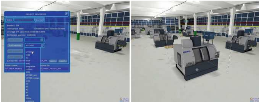
Fig. 12.6 Selecting a machine template from the GUI and placing it on the factory floor
