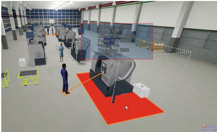
Fig. 12.8 Simulation data displayed in the Virtual Factory. Note the area around the bottleneck machine
