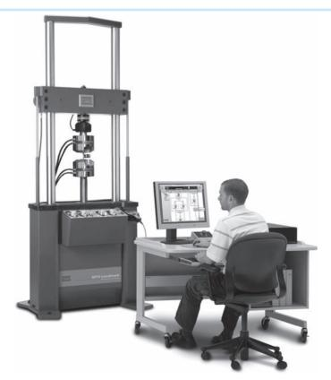
are then converted to stress and strain by using Equations (5.2) and (5.3). When the stress–strain data is drawn on a graph, the slope in the low-strain region is measured to determine E, and the value of the stress  $S_y$  at the yield point is read off the curve.
