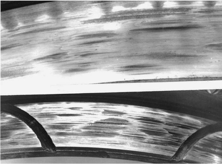
Fig. 9.18. Scuffing and thermal streaks on the friction cone of a commercial vehicle synchronizer hub
