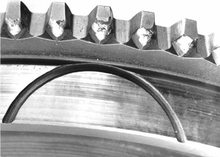
Fig. 9.16. Damage to the dogs of the selector teeth caused by grating. Ring groove in the friction cone of the commercial vehicle synchronizer hub
