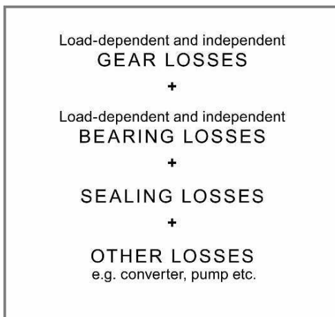
Fig. 2.32. Composition of losses in vehicle gearboxes
