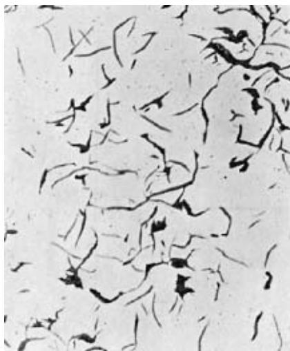
Fig. 6.3.2 Gray iron with flake graphite. Unetched, 100×.
