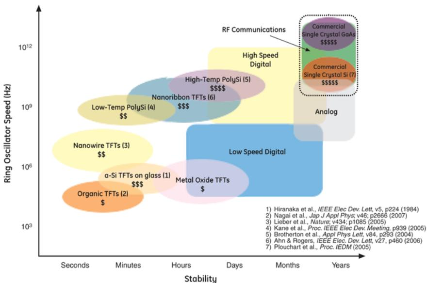
Figure 27: Device Speed and Stability Specifications
