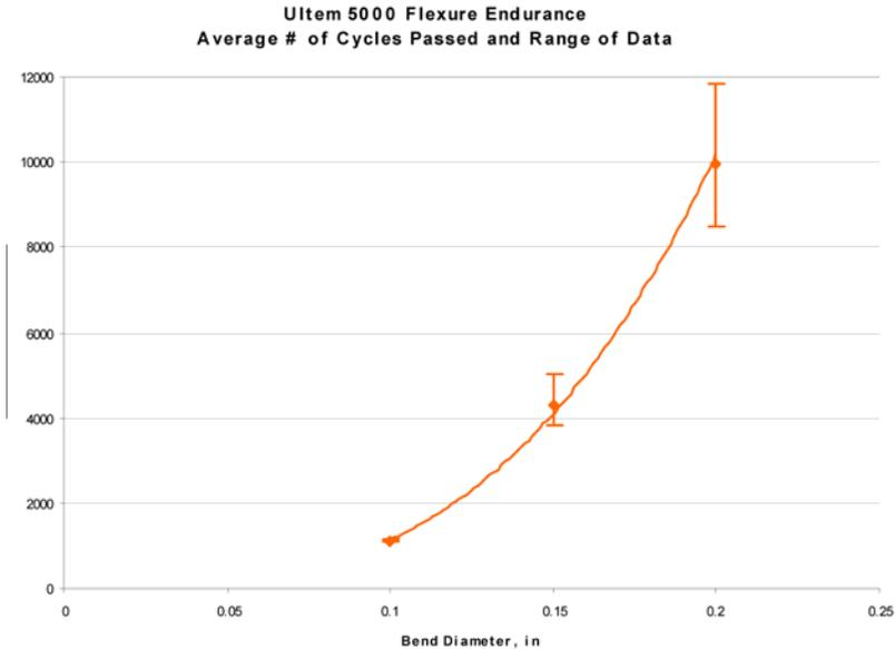
Figure 11: Example of Data Output from GE Research Flexural Endurance Tester (Utem polyimide film characterization)
