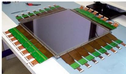
Figure 23: GE Digital X-Ray Detector Assembly
