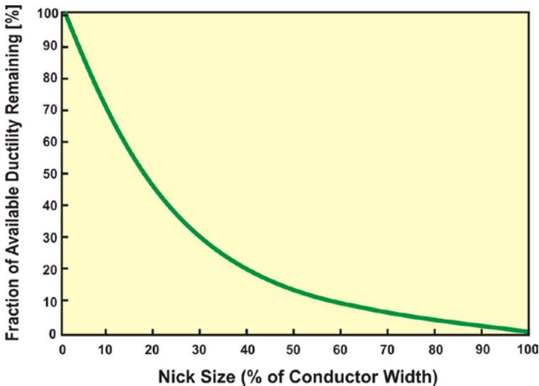
Figure 6. Reduction in Available Ductility Due to Conductor Defects.
