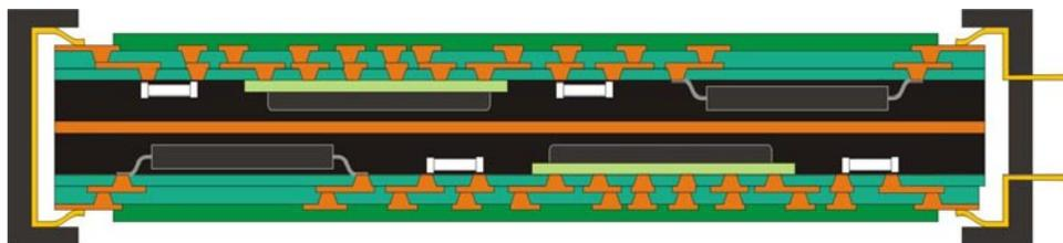
Figure 4: Components can be embedded in both face-up and face-down manner and attached to a central heat spreader, as shown. Connections from side to side can be made with connectors, as shown, or with through-hole "via plugs" that can be placed where needed on the assembly, another when possible and desired for even higher density designs.
