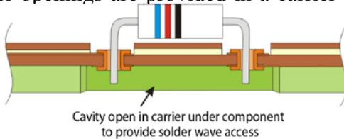
Figure 7-3. Fixtures for wave soldering should support the flex circuit through the wave while providing access to the leads and through holes of the flex circuit. The edges of the pallet wall should be chamfered as much as possible to allow the solder to flow in and out from the aperture. Ideally, the gap between the lead and the edge of the pallet on the trailing edge should be larger to aid solder drainage.
