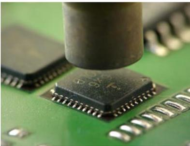
Example of the Land Grid Array (LGA) package being reworked on a polyimide flexible circuit with a hot air tool.
