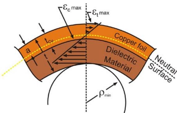
Fig. 3 Strain Distribution in Bent Single-Sided Flexible Printed Circuit Wiring
