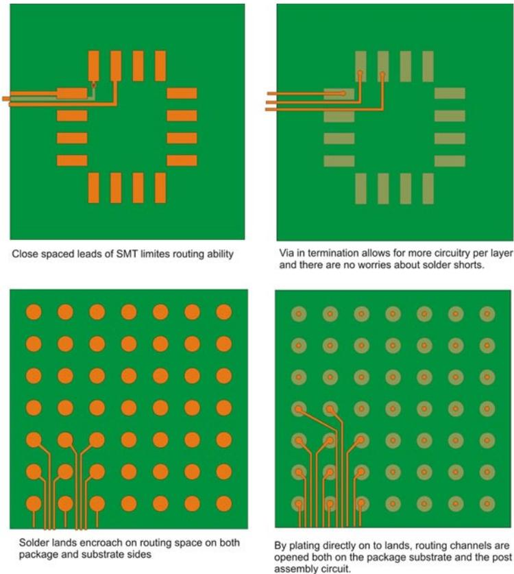
Figure 6: Routing advantages are possible for both peripheral and area array packages. Moreover, because there is no need for reflow and cleaning, the Occam process allows for edge-to-edge tiling of BGAs to create shorter path interconnections with reduced energy use and higher performance..
