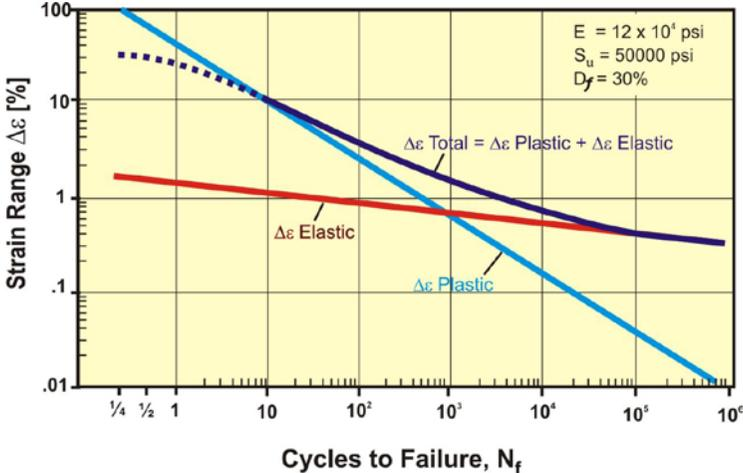
Figure 4. Strain Range-Fatigue Life Curve for Electrodeposited Copper
