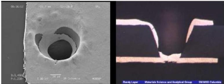
Figure 7: SEM and Cross-sectional Images of Incomplete Via Plating
