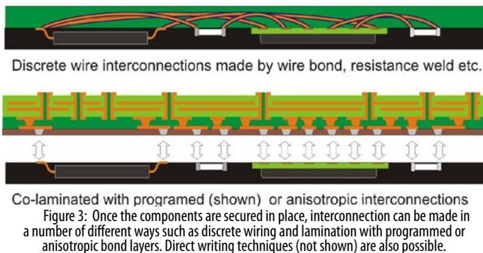
Assemblies of this type are expected to be low in cost and readily adaptable to the integration of thermal enhancements such as internal heat spreaders or even heat pipes, as well as EMI shielding, embedded electrical and optical components, and more.
