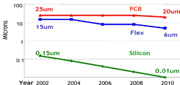
Figure 12: Silicon, Flex and PCB Minimum Feature Comparison
