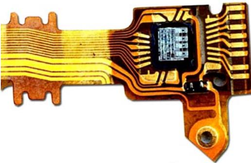
Figure 7-10 Example of a chip-on-flex assembly in which the IC chip is wire-bonded directly to the flex circuit. (Courtesy Interconnect Systems, Inc.)
