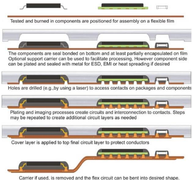
Figure 9: The Occam process applied to flexible circuits offers some unique design and assembly possibilities.
