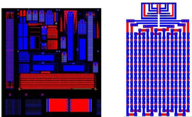
Figure 5: Test Element Group Design, Via String Coupon
