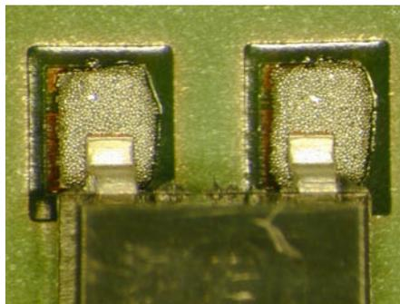
Examples of components placed onto solder paste prior to reflow; the two examples show a row of terminations on a Land Grid Array and SOT23 package. (Photo courtesy of Bob Willis)
