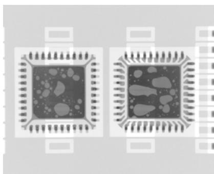
X-ray images of gull wing and LGA terminations assembled with tin-silver-copper were inspected and captured in real time on a DAGE system. (Courtesy of Bob Willis)
