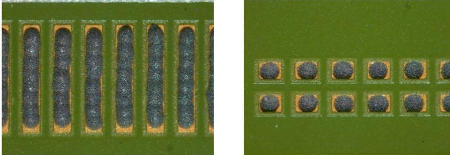
Examples of solder jetting being used on a circuit board for fine pitch and 0201 chip components. The circular pattern of the round jetting patterns is just visible in the surface of the paste. The images were taken from a board process on a Mydata MY500. (Courtesy of Bob Willis)
