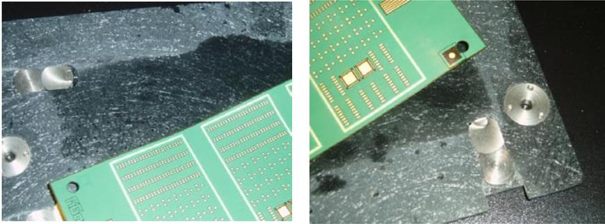
Using support pallets with vapor phase soldering requires modification to prevent the fluid being retained under the circuit. Holes placed under the circuit will reduce dragout of the fluid. (Photos courtesy of Bob Willis)
