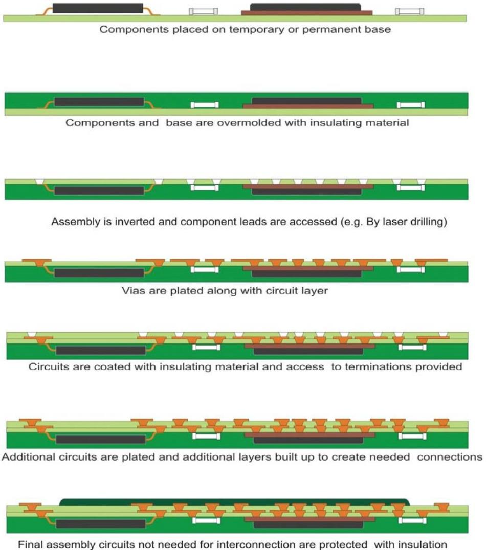
Figure 1: The basic Occam process manufacturing steps.
