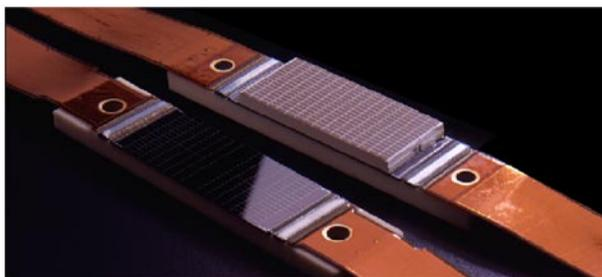
Figure 17: 4-Slice CT Detector Modules
