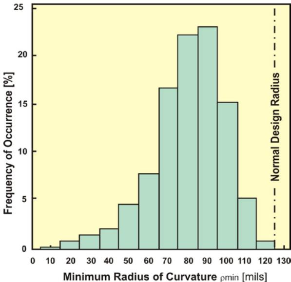
Fig. 5 Observed Minimum Radius of Curvature Distribution for Formed FPW with a Nominal Design Radius of 125 mils.
