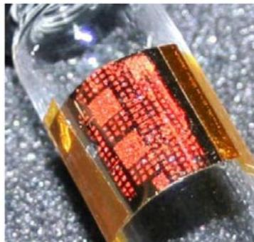
Figure 25: Printed Circuit on Curved Surface (Image courtesy of Alejandro Briseno/Stanford University)
