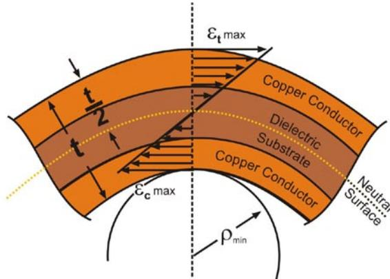
Fig 2: Strain Distribution in Bent Symmetric, Double-Sided Flexible Printed Circuit Wiring
