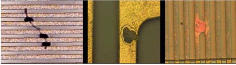
Figure 1: Examples of Flexible Printed Circuit Defects
