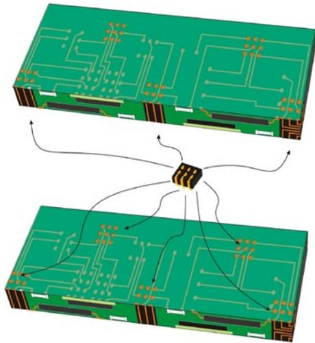
Low profile connectors such as above make connections between assemblies. They can be discrete as shown or in sheet form. A layer of material with cutouts for connectors and their alignment can be provided.
