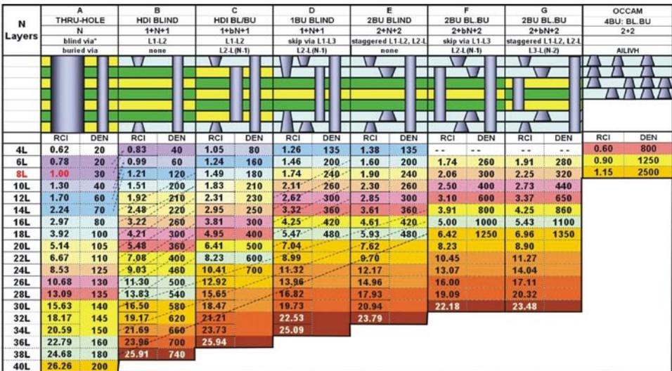
Figure 8: A spreadsheet analysis of relative cost of various multilayer circuit constructions and the I/O density capability reveals that, when compared to a standard 8-layer plated-through-hole construction having a relative cost of 1.0 and I/O density of 30 pins per square inch, an Occam buildup structure is capable of replacing up to a 14~18-layer board while providing 2500 I/O and maintaining a relative cost of 1.15. (Data and graphic courtesy of Happy Holden, Mentor Graphics)
