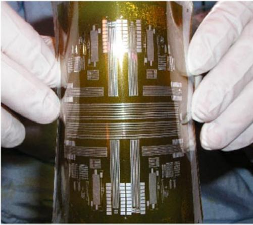
Figure 116: 4 $\mu$ m-Pitch Flexible Printed Circuit
