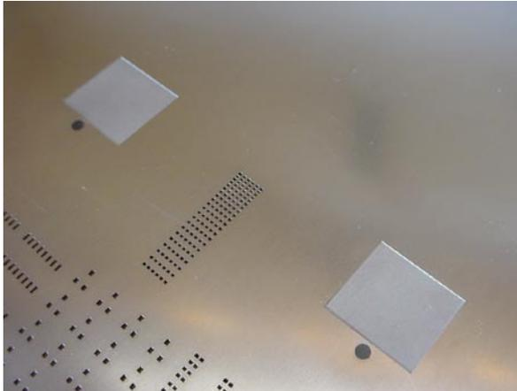
The base of this solder paste stencil foil has been designed to allow for minimum pin protrusion during the printing process. (Photo courtesy of Bob Willis)
