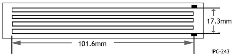
Figure 9: Flexural Endurance Test Pattern
