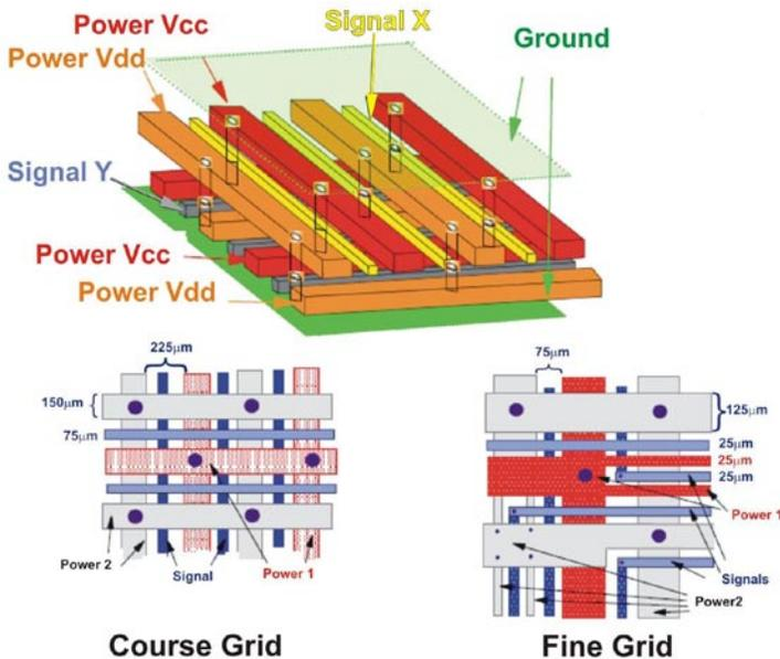
Figure 7: The Occam process is well suited to designing with the IMPS approach developed at the University of Arkansas, or the similar Power Grid concept developed at HP, which employs full metal grounds. Significant layer reductions can be achieved. With Power Mesh, multilayer routing efficiency for each layer approaches 95%. (Image courtesy of Happy Holden, Mentor Graphics)
