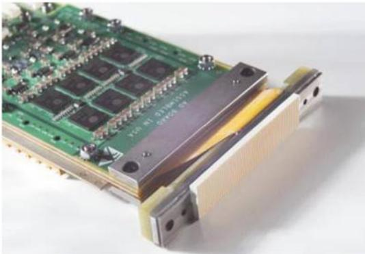
Figure 18: GE LightSpeed VCT Detector Module
