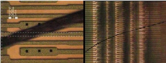
Figure 3: Defects in Two-Metal-Layer Flex
