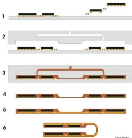
Figure 10: Injection molding allows for monolithic assembly and the integration of component stiffener and flexible interconnections according to the following plan: 1) Place components in mold; 2) Clamp mold; 3) Injection mold components in situ including strain reliefs; 4) Remove from mold; 5) Form metal circuits and coat with insulator material; 6) Form to desired shape.
