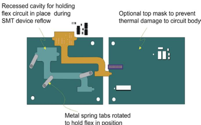
Figure 7-4. The fixture for surface mount on flex serves to keep the circuit flat and supported during the reflow operation. A top mask can be employed to prevent thermal damage to the bulk of the circuit. This facilitates the soldering of lower melt temperature base materials when they are economically preferred.
