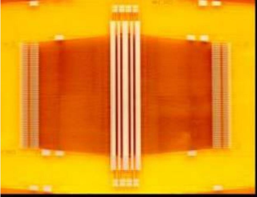
Figure 4: Ultrasound Flex Circuit
