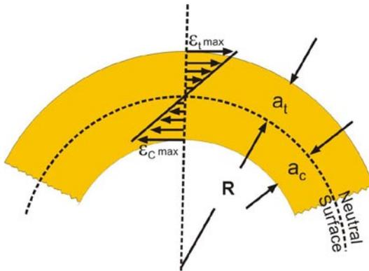
Fig. 1: Strain Distribution in a Bent Beam
