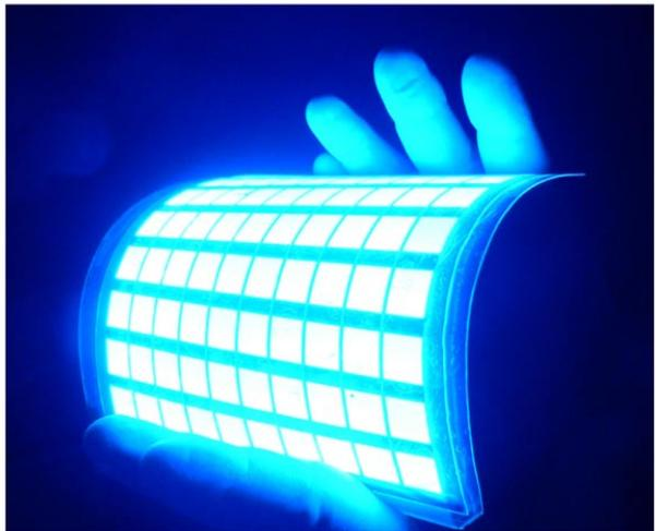
Figure 26: Printed OLED Array
