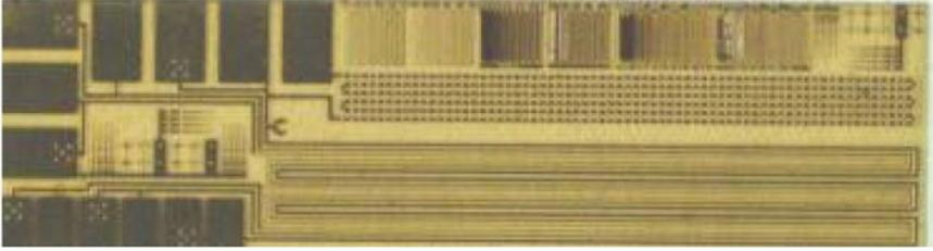
Figure 10: GE Fine-Pitch Flexural Endurance Coupon (array of trace pitch, 1-metal-layer vs. 2-metal-layer design)
