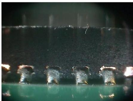
These examples show typical lead-free solder joints on a flexible circuit after assembly and soldering. Examples of a gull wing lead on an SOIC and LGA terminations were captured with an ERSA Scope. (Photos Courtesy of Bob Willis)
