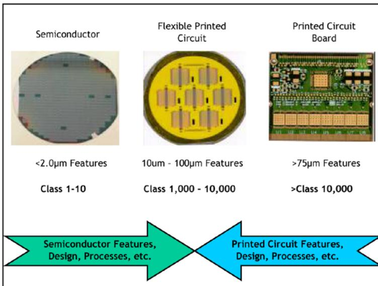
Figure 2: Semiconductor, Flex, and PCB Comparison
