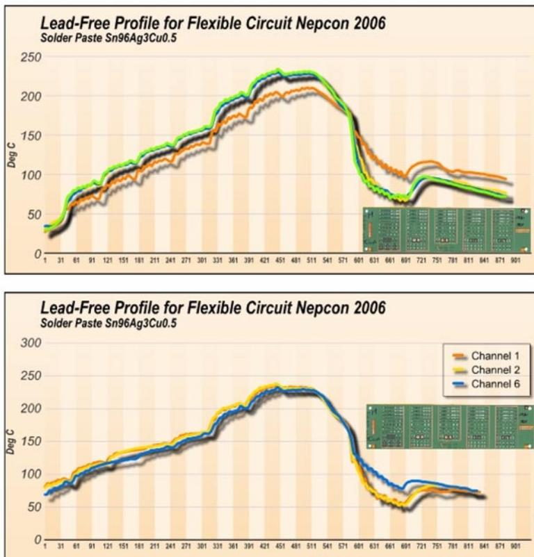
Figure 7-8: Two lead-free soldering profiles for a flex circuit assembly on a process carrier using a KIC profiler. The first profile shows a larger delta T between selected terminations on the circuit. After modification to the carrier and reduction of the thermal mass, the second profile shows a more acceptable reflow profile. (Courtesy of Bob Willis)
