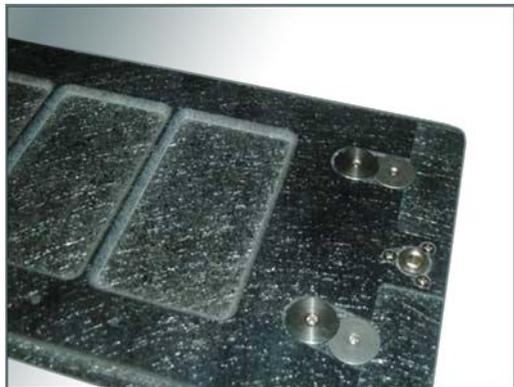
Figure 7-5. Example of a carrier for flexible circuit assembly. Thermal relief areas on the base of the pallet have been machined directly under the active circuits to improve delta T during reflow. Also consider drain holes under the flex if using vapour phase reflow or if cleaning is being considered. (Photo courtesy of Bob Willis)
