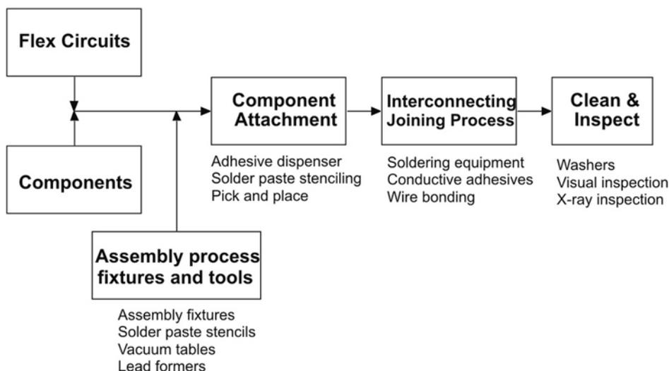
Figure 7-1 Simplified flow diagram for flex circuit assembly
