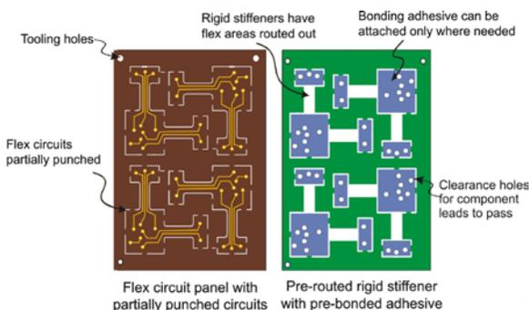
Figure 7-2. Mass application of stiffeners in panelized form facilitates both stiffener application and component assembly. When bonded together, the circuit can be processed much like a rigid board.
