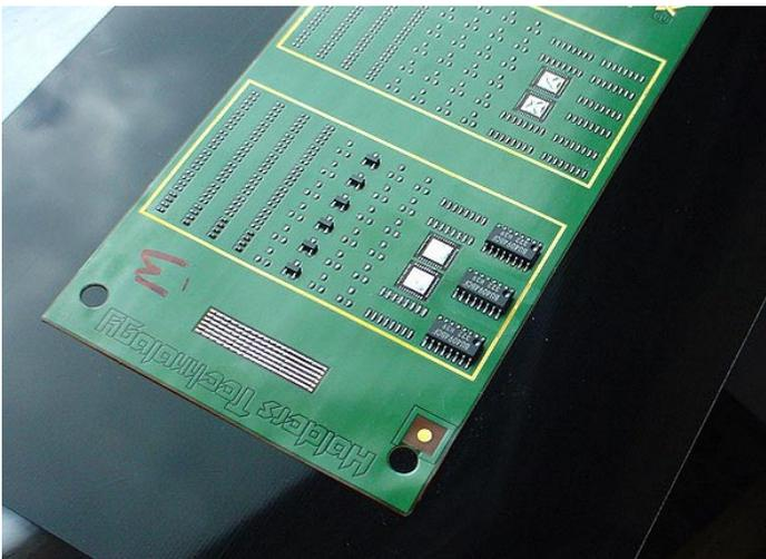
Example of a sticky pallet with a flexible circuit assembly in position. Normally, the sheet of material would have some tooling holes to make automatic placement of the flexible circuits possible in production. (Photo courtesy of Bob Willis)
