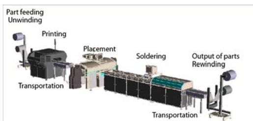
Figure 7-9 A prospective piece of equipment for reel-to-reel assembly of flexible circuits. (Source: Siemens L&A)
