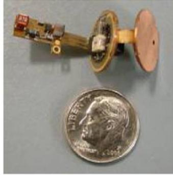
Figure 22: LNA-Balun Flex Assembly
