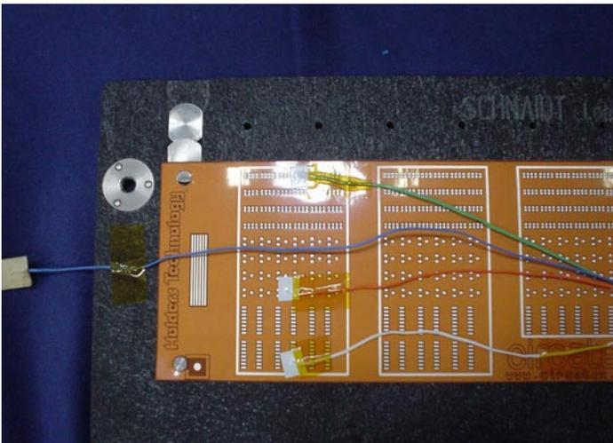
Profiling a flexible on a pallet may require a combination of thermocouple attachment techniques. The use of high-temperature solder is the preferred technique, but aluminum tape can be very beneficial on flexibles. The pallet was set up for profiling with an air probe for the KIC system. (Photo Courtesy of Bob Willis)
