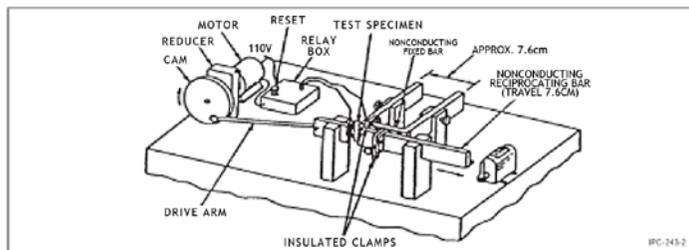
Figure 8: Flexural Endurance Tester per IPC
