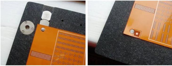
Figure 7-6. Zero standoff pins serve for aligning and holding the flex circuit to the fixture. Any minor protrusion of the pin above the surface of the flex would need to be considered in the solder paste stencil design. (Photos courtesy of Bob Willis)
