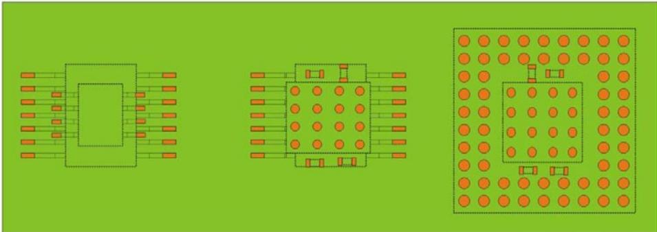
Component contact view of cross section above show land patterns for packaged IC components and discrete devices.
