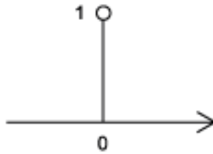
Figure 2.36: The graphical representation of the discrete-time impulse function
