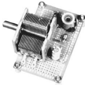
1-7 VFO circuit build on perfboard.
