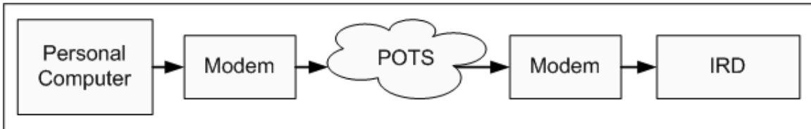
Figure 8-15 IRD control via a PC
