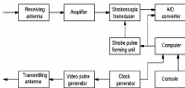
Figure R32 Impulse radar with ultrawideband signal.
