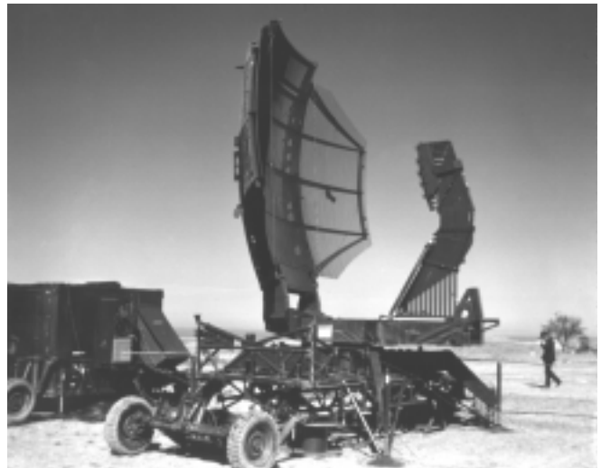
Figure A76 AN/TPS-43 stacked-beam reflector antenna.
