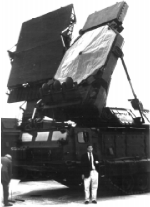
Figure F17 The SA-12 Grill Pan fire control radar, an example of a space-fed lens array. In the background is the Billboard three-dimensional surveillance radar.
