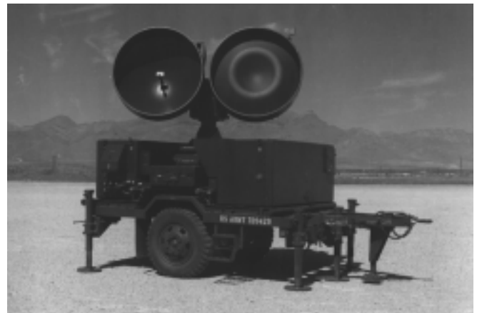
Figure R18 AN/MPQ-46 tracking illuminator for the Hawk missile system (Raytheon photo).
