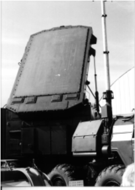
Figure R24 SA-10 Flap Lid fire control radar for the SA-10 SAM system.
