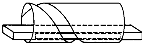
Figure S7 Helical-slot scanner (from Johnson, 1984, Fig. 18.29, p. 18.25, reprinted by permission of McGraw-Hill).
