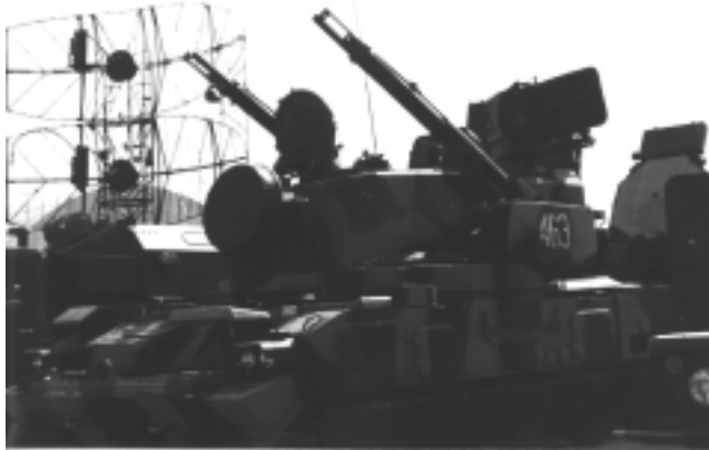
Figure R21 Russian anti-aircraft gun and missile system, using S-band search and K_u -band fire control radar.
