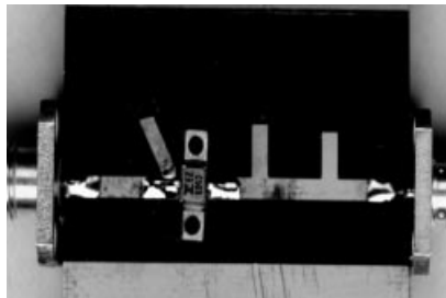
Figure 6.14. (a) Approximate Class E power amplifier circuit in which the transistor is represented as an ideal switch, and transmission line sections are used for the output match and harmonic tuning. (b) Hybrid implementation with single stub.
