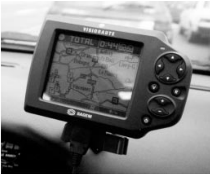
Figure 7.15 The Sagem/Médiamobile Visionaute is designed for a pay-service in Paris using the ALERT-Plus with the ALERT-C protocol. (Source: EBU.)
