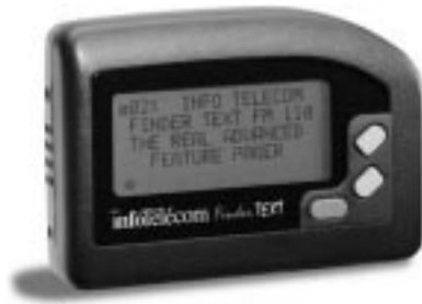
Figure 8.4 The 1997 model RDS FM 110 of a new pager from Info Telecom in France, permitting reception of 80 alphanumeric character messages. (Source: Info Telecom.)
