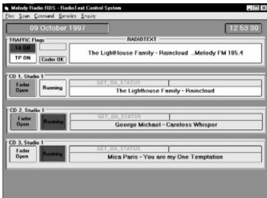
Figure 4.5 RadioText computer display: showing on-air RT messages and those cued for transmission. (Source: EBU.)
