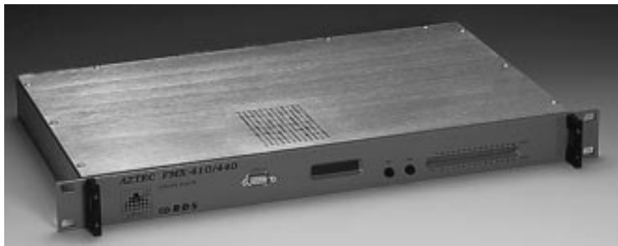
Figure 11.1 First RDS encoder implementation of UECP version 5.1: the AZTEC RADIOMEDIA FMX 440 Digiplexer (RDS and DARC). (Source: EBU.)
