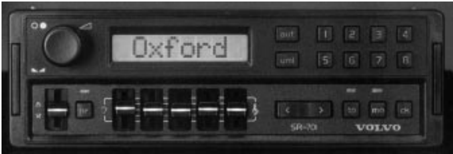
Figure 1.6 In 1987, the Volvo 701 first commercial RDS car radio in the world. (Source: Volvo.)
