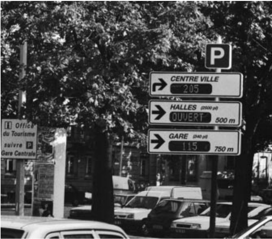
Figure 7.22 Car park status information in Strasbourg updated via RDS-ODA. (Source: Info Telecom.)
