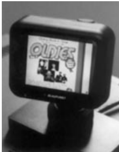
Figure 13.3 DAB makes it possible to implement multimedia services on DAB. During a 1997/98 field trial in Germany, SDR/SWF used the MOT protocol to broadcast pictures with CD covers of pop music titles on air. (Source: EBU.)
