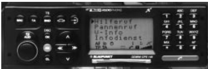
Figure 7.17 Blaupunkt integrates in the GEMINI a car radio, GSM and GPS. (Source: Blaupunkt.)
