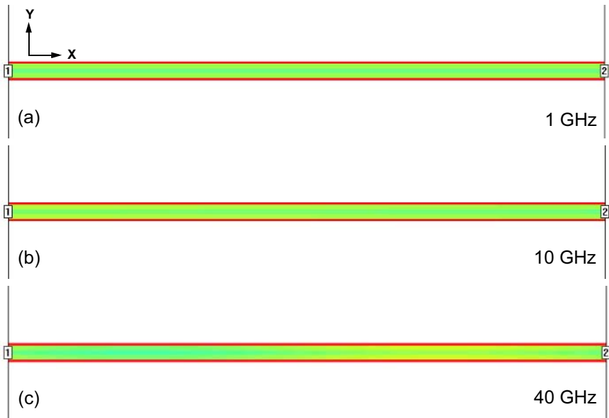
Figure 10.13 Conduction current, mostly X-directed, on a microstrip line on a gallium arsenide substrate: (a) current at 1 GHz, (b) current at 10 GHz, and (c) current at 40 GHz. The scale is 0 to 300 amps/meter (Sonnet em Ver. 7.0).
