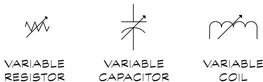
Figure 6-8: Schematic symbols for variable components use an arrow or other mark to show that the value of the component is changeable.
