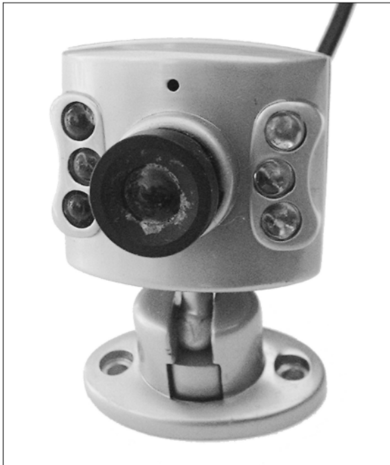
Figure 14-6: This miniature camera can see in the dark, thanks to its six infrared-emitting diodes.
