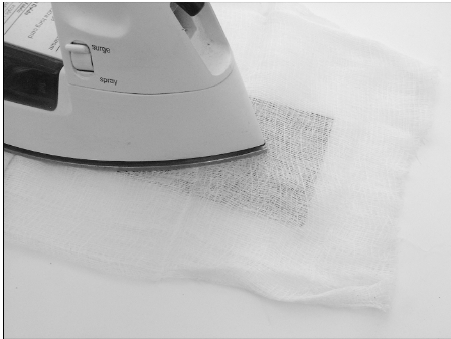
Figure 12-5: Use a clothes iron to transfer the toner from the transparency to the copper clad.
