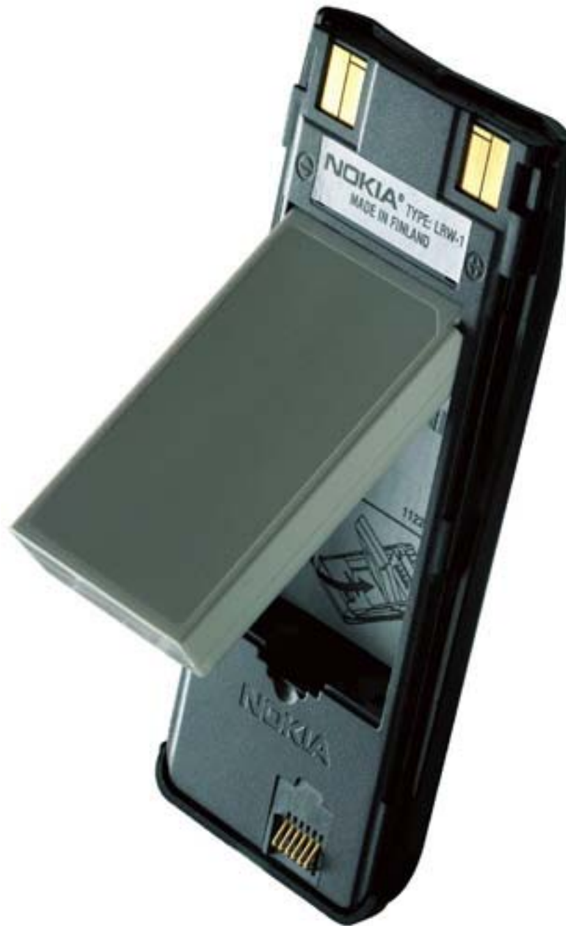
Figure 5.10: Nokia's Connectivity Battery adds Bluetooth functionality to their model 6210 cellular phone. (Photo courtesy Nokia Corporation)
