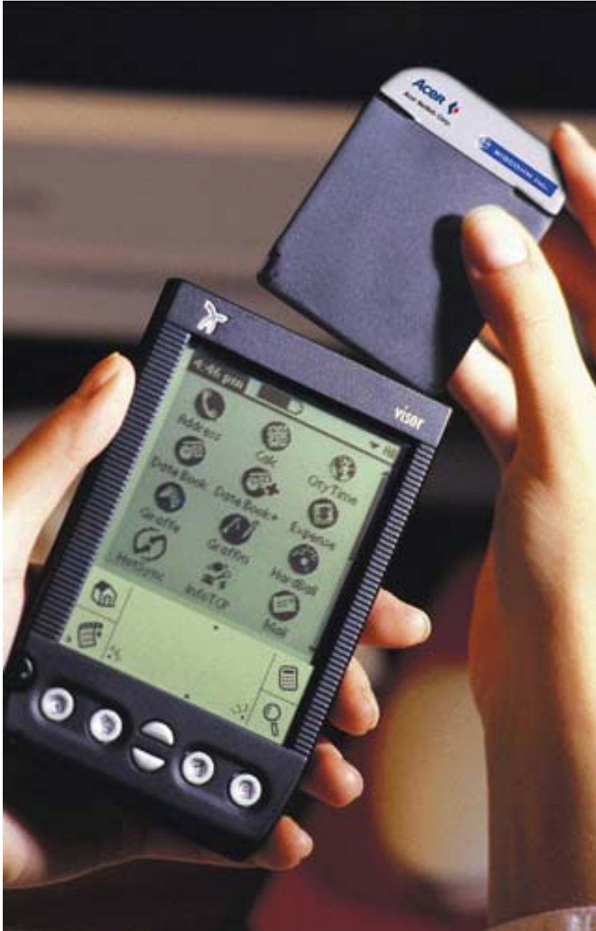
Figure 5.4: Acer's Blue-Connect module adds Bluetooth functionality to the Handspring Visor. (Photo courtesy Acer NeWeb)
