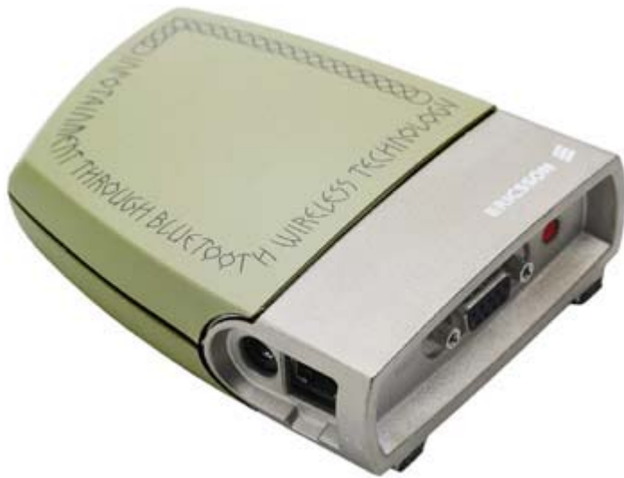
Figure 5.22 : Ericsson's BLIP access point base station/server (Photo courtesy Ericsson)
