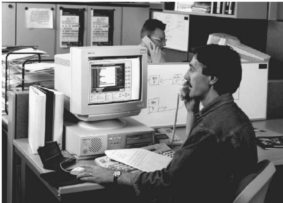
Figure 5.9 A typical display on the PC screen of a virtual remote test system. The front panel of the remote test set is replicated at the controlling PC. The front panel can be operated by pointing and clicking the mouse, while the displayed results from the remote tester are relayed back to the PC and appear as they would at the remote site. Virtual remote systems allow both ends to control the test set for maximum flexibility when troubleshooting.
