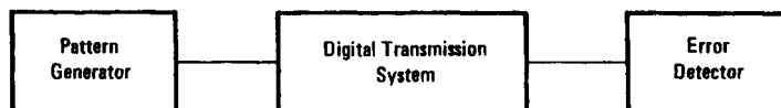
Figure 26.3 To test a digital transmission system, a pattern generator is connected to the input of the system under test, and an error detector is connected at the output.
