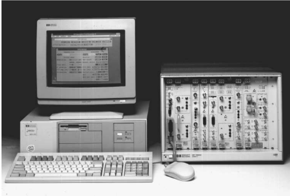
Figure 30.11 Typical “leading-edge” R&D analyzer ( courtesy Hewlett-Packard ).
