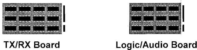
Figure 18.10 Cellular phone modules. Keyboard, battery, and antenna would be completely replaced if faulty. The circuit boards usually are repaired down to the component level. This might happen at the service shop if it is suitably equipped, or the circuit boards might be exchanged in a parts pipeline process with the manufacturer.
