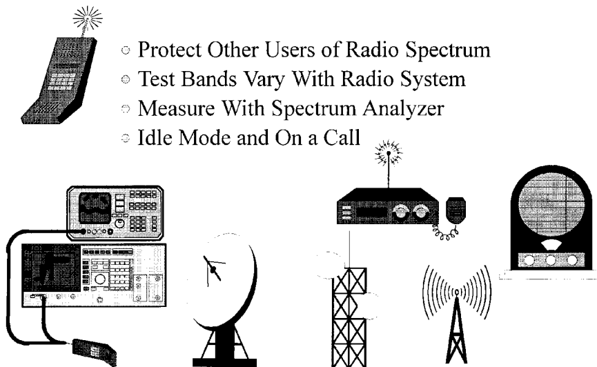
Figure 19.4 Spurious emissions. These are measured with a spectrum analyzer. The test frequency bands will vary depending on the radio system. Any unplanned or unwanted RF signals generated by the transceiver device are designated as spurious.
