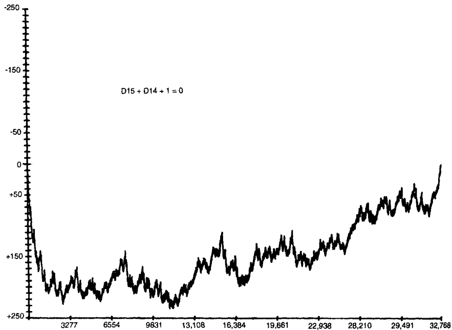
Figure 26.8 This graph shows the running digital sum for a commonly used PRBS. Notice the initial steep descent of the graph, indicating a predominance of 1s or 0s (depending on inversion) for the initial period of the sequence.
