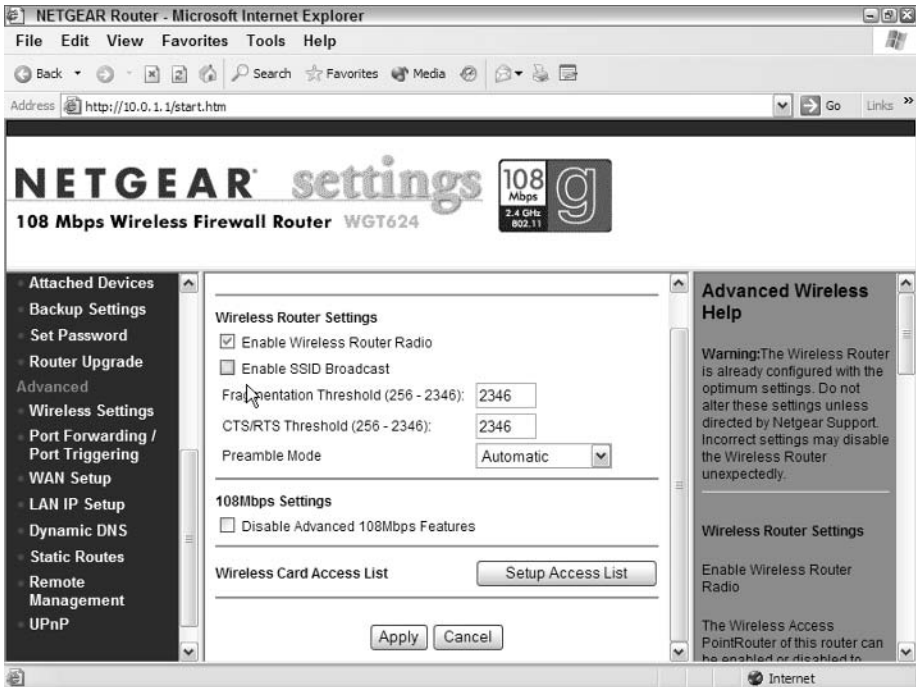
Figure 16-3: Turning off the SSID broadcast helps hide your network.
