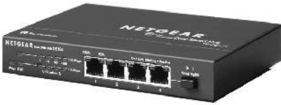
Figure 14-5: A Netgear wiring hub.
