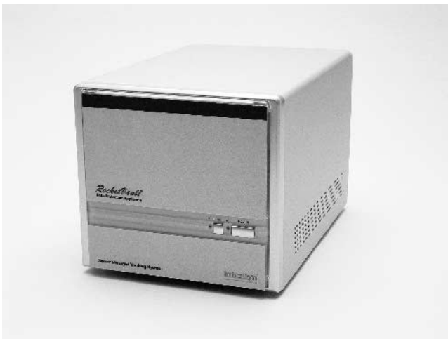
Figure 13-12: RocketVault is built into a Shuttle PC case.
