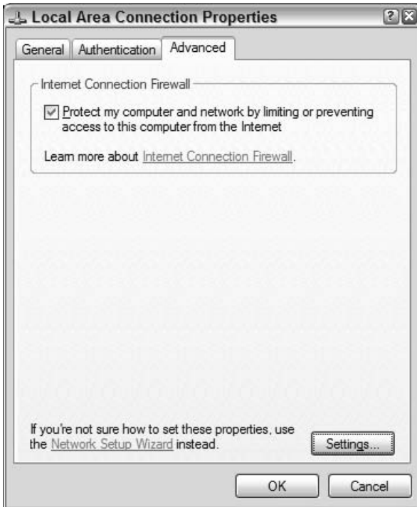
Figure 11-19: Turn on your Internet Connection Firewall if you have no network router with firewall capabilities.
