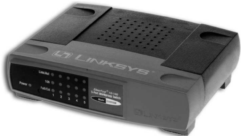
Figure 14-6: A Linksys five port switch for home and small office use.
