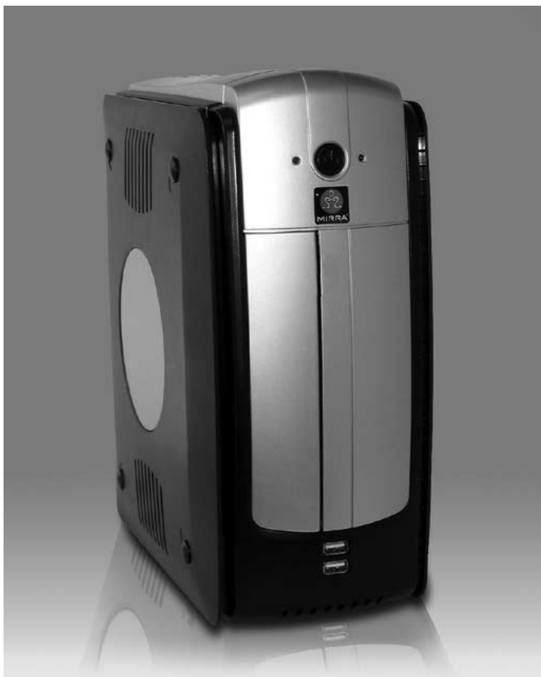
Figure 13-8: A combo system: backup and remote sharing device, the Mirra Personal Server.
