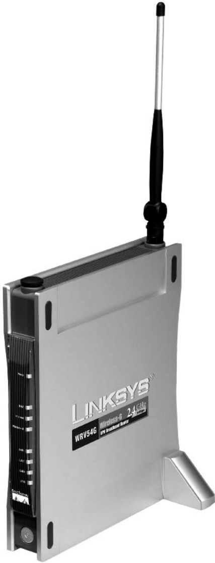
Figure 8-3: An updated Linksys router with Ethernet and advanced wireless networking options
