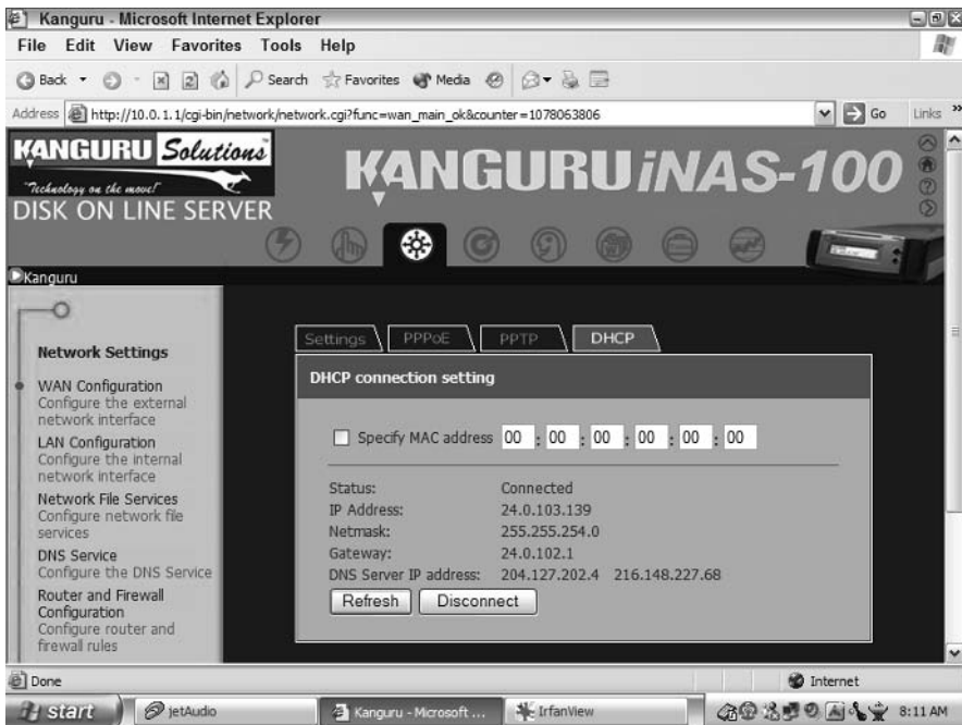
Figure 12-3: Notice the DNS Server IP address listing at the bottom of the screen.
