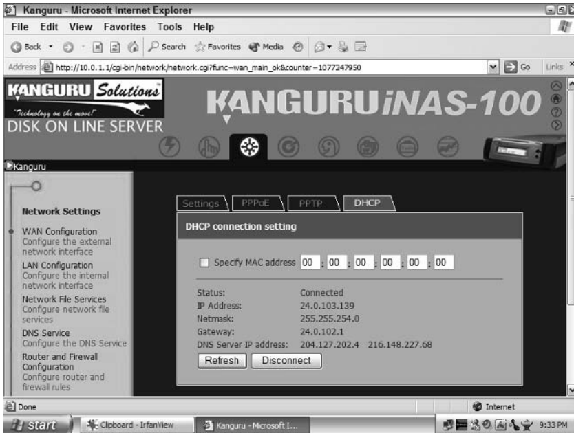
Figure 10-17: The Kanguru router as DHCP client to a cable modem.
