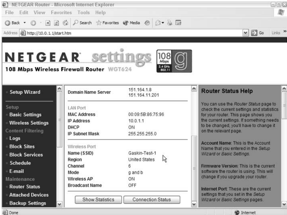
Figure 16-2: Wireless port configuration status screen for the Netgear WGT624.
