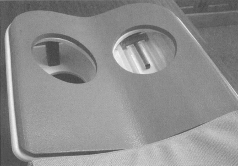
Figure 3. Clinical MRE imaging apparatus with breast coil and mechanical actuator (on right-hand side).
