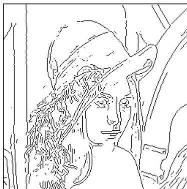
Figure 11.12: Edge chains calculated from wavelet transform modulus maxima at the finest scale. The longer chains are shown.
