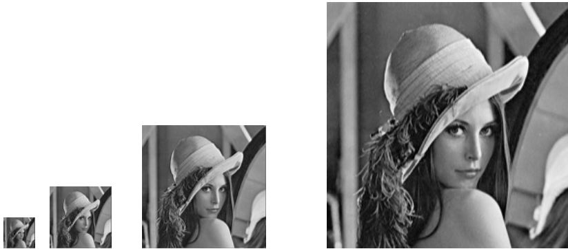
Figure 7.23: Multiresolution approximations a_j[n_1, n_2] of an image at scales 2^j , for -5 \geq j \geq -8 .
