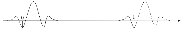
Figure 7.18: The restriction to [0,1] of a periodic wavelet \psi_{j,n}^{\text{per}} has two disjoint components near t=0 and t=1 .
