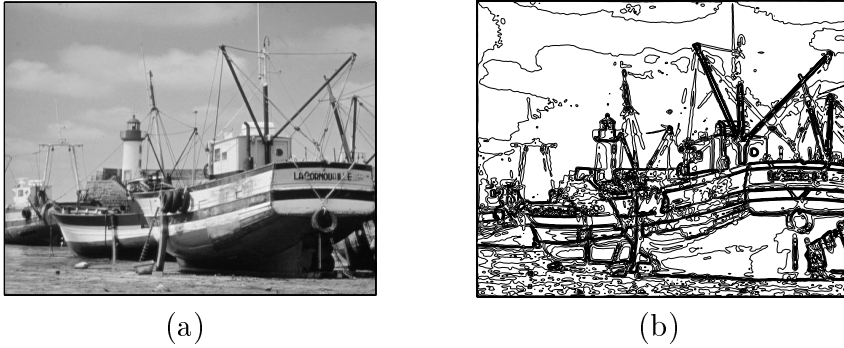
Figure 2.2: (a): The total variation of this image remains nearly constant when the resolution N increases. (b): Level sets \partial\Omega_y obtained by sampling uniformly the amplitude variable y .
