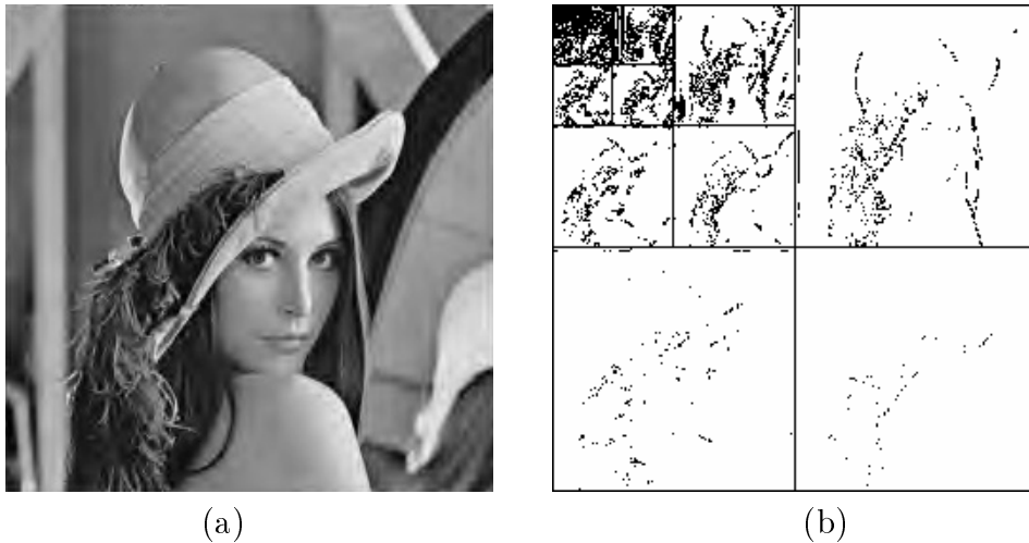
Figure 9.4: (a): Non-linear approximation f_M of a Lena image f of N^2 = 256^2 pixels, with M = N^2/16 wavelet coefficients: \|f - f_M\|/\|f\| = 0.011 . Compare with the linear approximation of Figure 9.2(b). (b): The positions of the largest M wavelet coefficients are shown in black.
