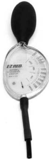
**FIGURE 7-22** Inexpensive plastic hydrometer for measuring specific gravity.
