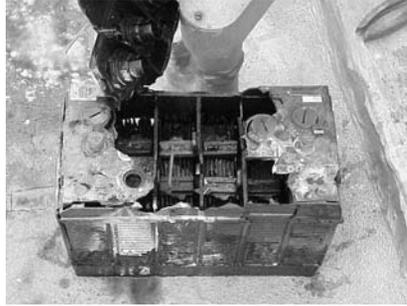
**FIGURE 7-25** Exploded battery. ([www.rayvaughan.com/images/battery/MVC-172F.jpg](http://www.rayvaughan.com/images/battery/MVC-172F.jpg))
