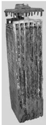
**FIGURE 7-14** Sulfation of battery plates. ([www.surfacematerials.com/Cell\\_sediment.jpg](http://www.surfacematerials.com/Cell_sediment.jpg).)
