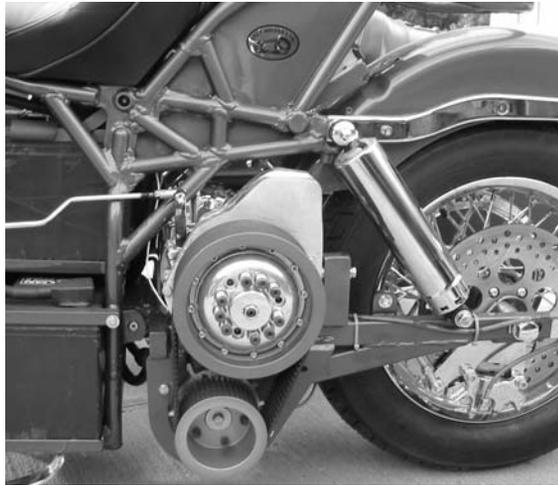
**FIGURE 13-14** Clutch basket and belt configuration.
