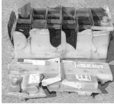
**FIGURE 7-24** Battery explosion resulting from gassing.
