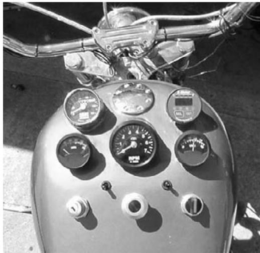
**FIGURE 11-1** Electra Cruiser prototype 1 tank gauge layout.
