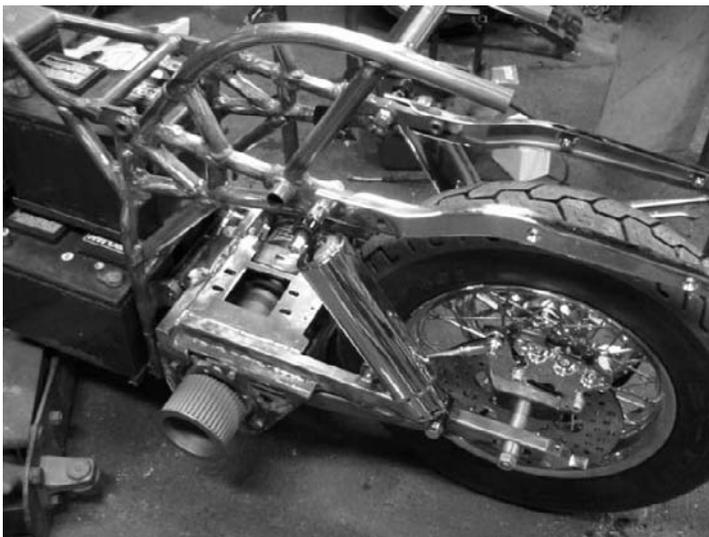
**FIGURE 13-12** Fitting the motor to the swingarm.
