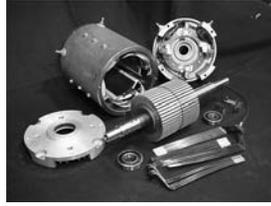
**FIGURE 8-5** Sample of basic dc motor. ([www.physclips.unsw.edu.au/jw/electricmotors.html](http://www.physclips.unsw.edu.au/jw/electricmotors.html).)
