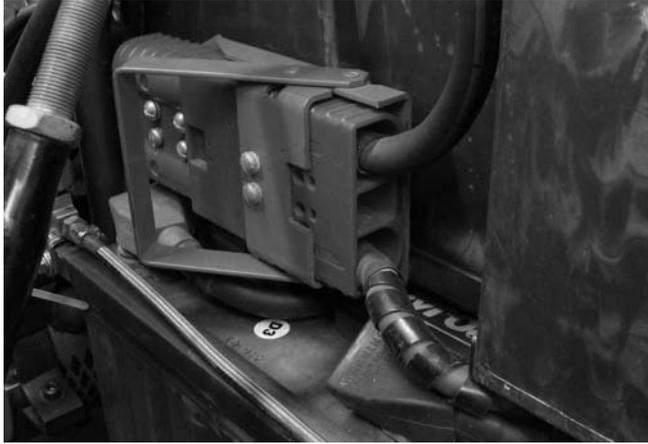
**FIGURE 12-2** Quick disconnect on the Electra Cruiser.
