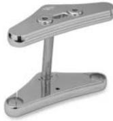
**FIGURE 5-10** Picture of a raked triple tree. (Courtesy of Custom Chrome, [www.customchrome.com](http://www.customchrome.com).)
