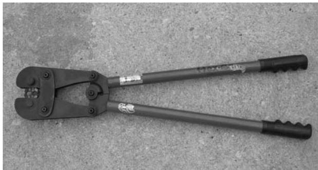
**FIGURE 12-9** Heavy-duty crimping tool.
