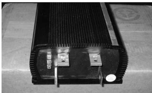
**FIGURE 9-16** View of Curtis Model 1231 series connections. ([www.curtisinst.com/index.cfm?fuseaction=cProducts.DownloadPDF&file=50003%5F1221C%2D1231C%5FRevD%2Epdf](http://www.curtisinst.com/index.cfm?fuseaction=cProducts.DownloadPDF&file=50003%5F1221C%2D1231C%5FRevD%2Epdf).)
