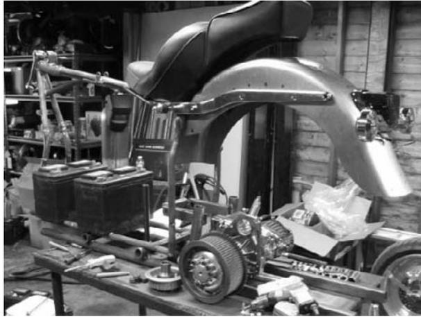
**FIGURE 13-7** Fitting the transmission to the swingarm.
