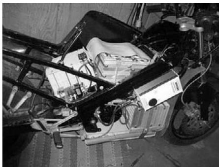
**FIGURE 4-2** Electrocat batteries and electric motor. ([evahakansson.se](http://evahakansson.se).)
