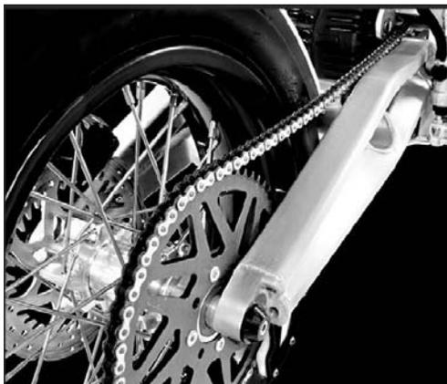
**FIGURE 13-9** ZERO electric motorcycle chain drive. ([www.zeromotorcycles.com/gallery.php](http://www.zeromotorcycles.com/gallery.php).)
