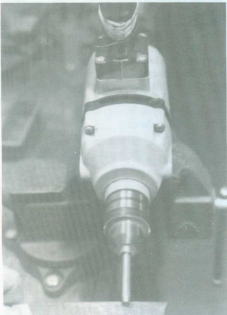
Wrap tape around bolt threads and chuck into fastened-down 1/2" drill. Work the end down to 1/16" for the firing pin.
