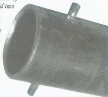
Completed M203 barrel with locking studs welded in place (left).
