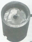
The 1 1/2" steel pipe piece dropped in breech as spacer, with firing pin washer dropped in on top of welded washer-spacer and second washer.
