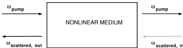
FIGURE 19 Backward stimulated scattering in which the scattered radiation propagates in the direction opposite to the pump radiation. The scattered wave either can be supplied along with the pump radiation, or can be generated from noise in the interaction.
