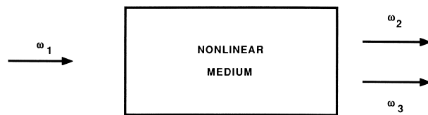
FIGURE 7 Schematic illustration of the waves used in parametric down-conversion. Radiation at \omega_1 is supplied, and radiation at \omega_2 and \omega_3 is generated in the nonlinear interaction.
