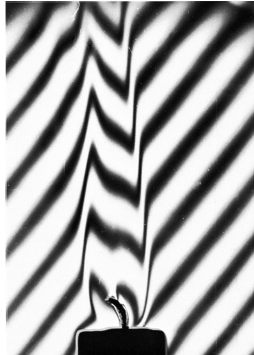
FIGURE 7 Shearing (schlieren) interferogram of the hot gases rising from a candle flame. (Photographed by H. Vanheiden, Universität Essen, Federal Republic of Germany.)
