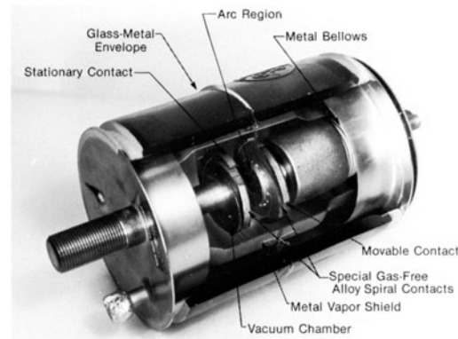
FIGURE 8 A modern 500-MVA vacuum interrupter.
