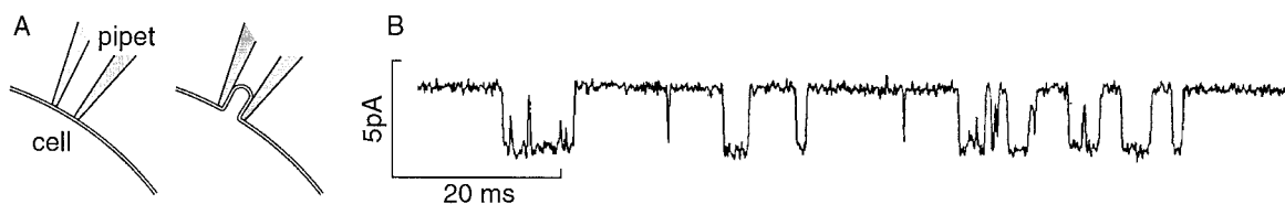
FIGURE 3 The single-channel current-recording technique. (A) The tip of a borosilicate glass pipet, with a tip opening of 1–2 \mu\text{m} is pressed against the membrane of a frog muscle cell (left). A slight negative pressure (20–30 cm \text{H}_2\text{O} ) is applied to the pipet for several seconds to form the seal between the membrane and the pipet (right). (Reproduced from O. Hamill et al. (1995). In "Single-Channel Recording," 2nd edition (B. Sakmann and E. Neher, eds.), p. 663, Plenum Press, New York.) (B) A typical current trace recorded using the single-channel technique, a rat myoblast cell containing nicotinic acetylcholine receptors, and 20- \mu\text{M} acetylcholine (pH 7.2, 22°C, and V_m = -80 mV). (Reproduced from F. Sigworth (1983). In "Single-Channel Recording," first edition (B. Sakmann and E. Neher, eds.), Plenum Press, New York.)
