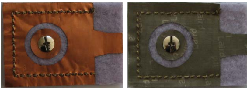
Figure 1.15 Textile-integrated slot loop antennas. Source: Based on data from Hubálek et al. 2016 [17].
