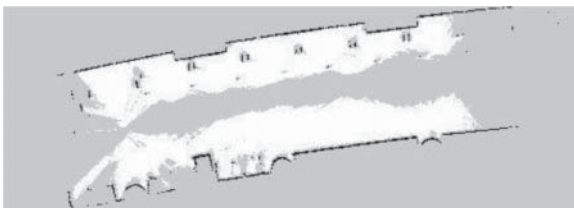
Figure 7.21 OGM of the Microwaves laboratory, ECE, utilizing Cartographer as SLAM algorithm.
