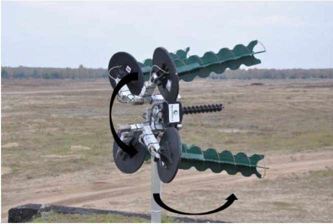
Figure 9.32 Tracking and data exchange system with indication of rotation planes.
