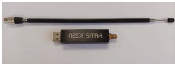
Figure 5.12 USB software defined radio receiver and telescopic monopole antenna for FM signals reception.
