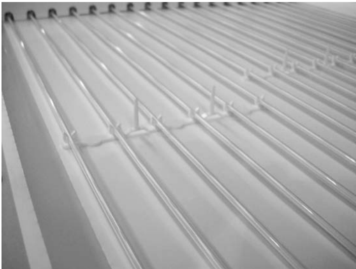
14.8 CCFL backlight array in the rear tray of an LCD television panel.
