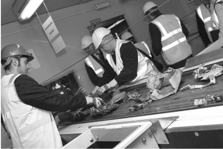
10.5 Photograph of a manual WEEE separation facility (image courtesy of SIMS Recycling Solutions).
