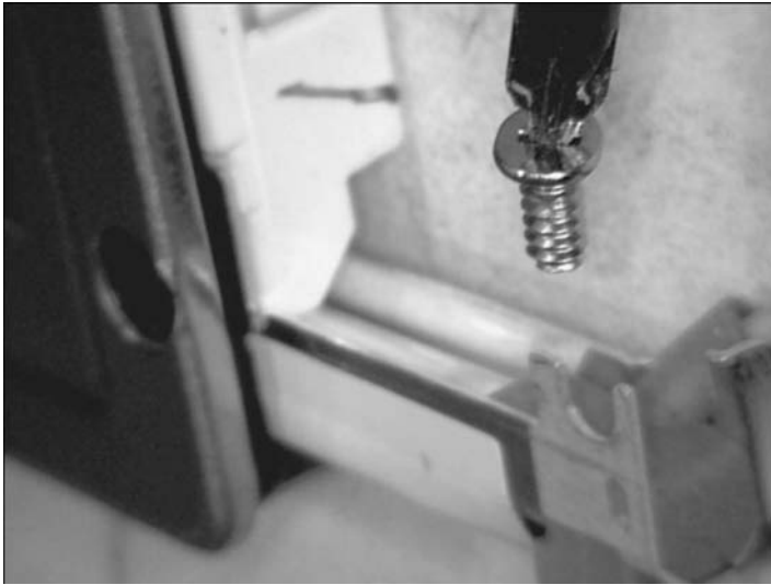
14.7 Removal of CCFL in metal carrier from a 15" monitor LCD panel.
