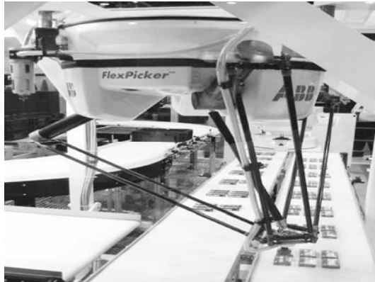
Fig. 1.3. The FlexPicker designed for industrial pick and pack of small lightweight objects, such as chocolates, with high speed. The cameras (not shown here) are integrated with the robot to identify and locate the object to be picked up
