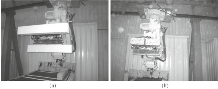
Fig. 7.51. Log unloading workcell. (a) Two logs coming out from a calciner conveyor are picked up by an inverted robot; (b) Two sets of grippers are mounted on the robot arm to pick up the log and three laser point sensors are mounted on each gripper to locate the log position and orientation
