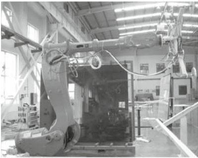
Fig. 7.58. Gripper with laser sensors is used to pick up solar panels
