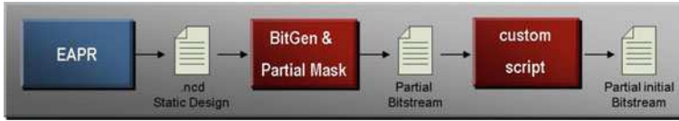
Fig. 17.6 Proposed flow for fast sequential startup using spartan 3 devices
