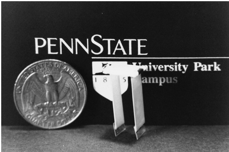
3.13 Two bimorph legs fixed to a plastic board.
