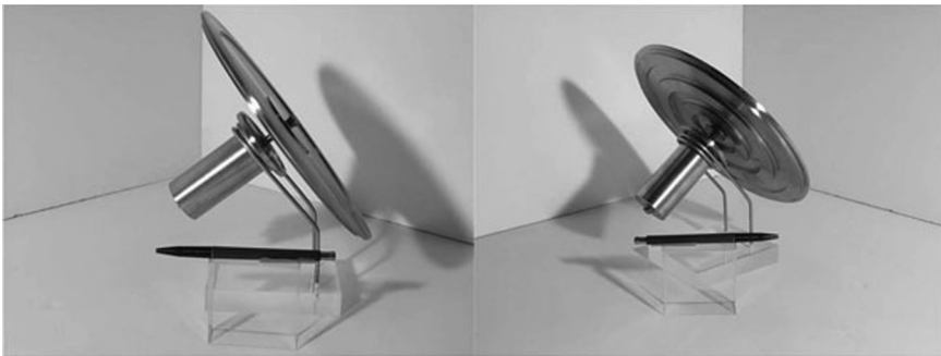
15.10 Prototype of a stepped-groove-plate transducer with an operating frequency of 41.3 kHz.
