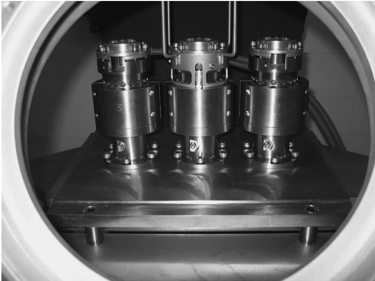
15.38 Semi-industrial reactor using rectangular grooved-plate power ultrasonic transducers for pigment dispersal in paints, pastes and inks.
