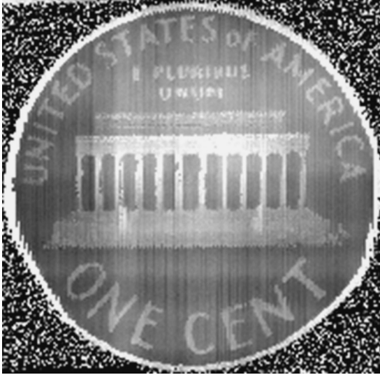
13.23 Ultrasonic front-surface image of a US one cent coin.
