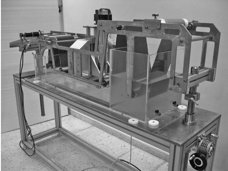
15.33 Semi-industrial implementation of ultrasonic textile washing.
