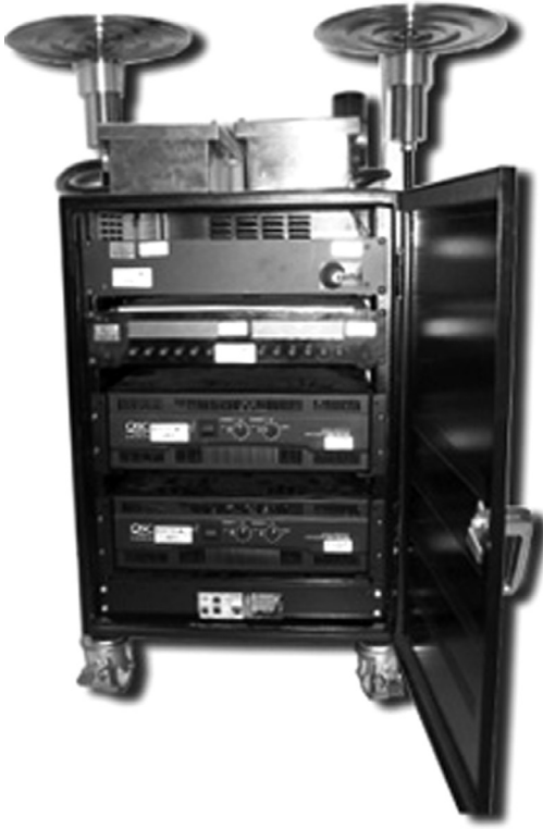
15.15 Ultrasonic defoamer system, which uses two stepped-grooved-plate transducers to focus airborne ultrasound.
