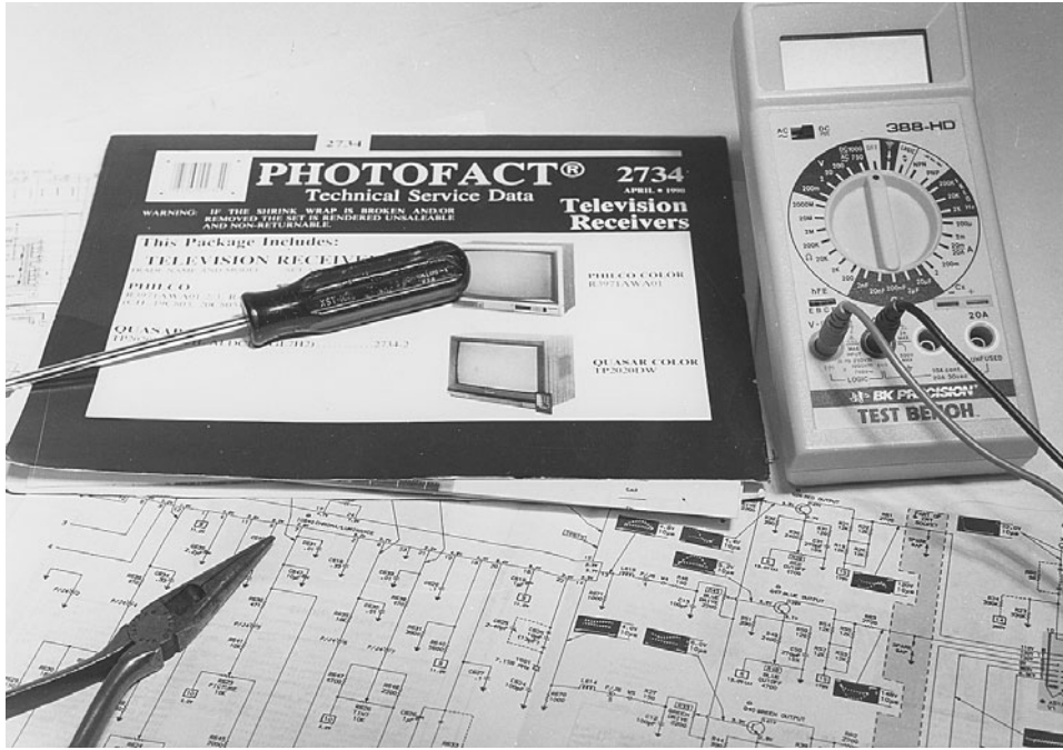
2-21 Sams Photofacts schematics can be used to check components in TVs and VCRs.
