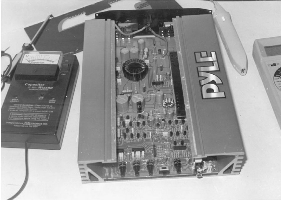
9-24 Check all electrolytics in the output audio circuits with an ESR meter.
