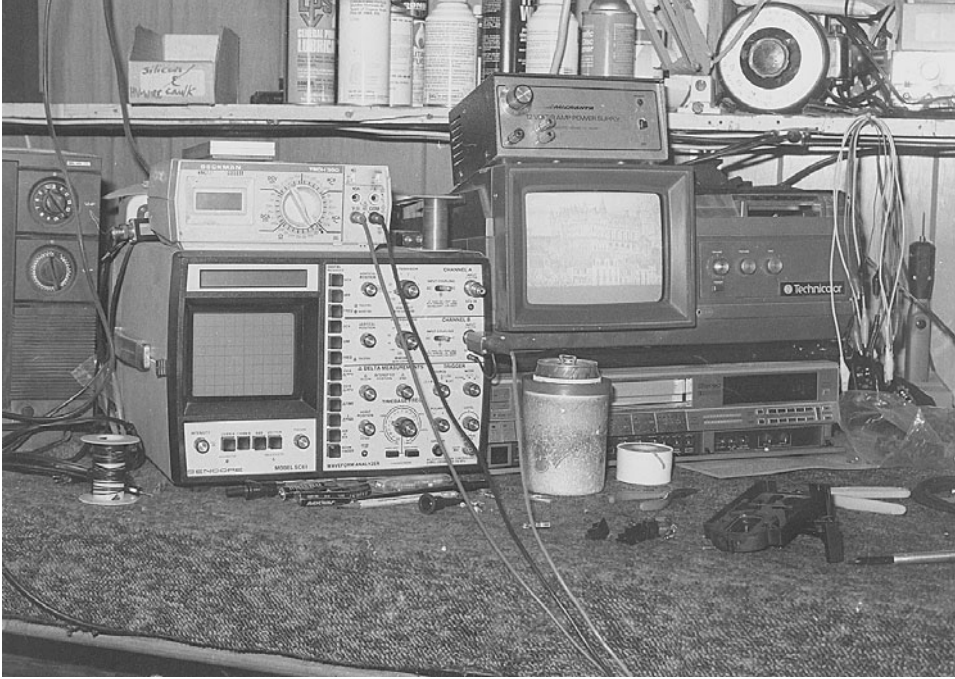
3-3 A frequency counter, scope analyzer, and external power supply are optional test equipment.
