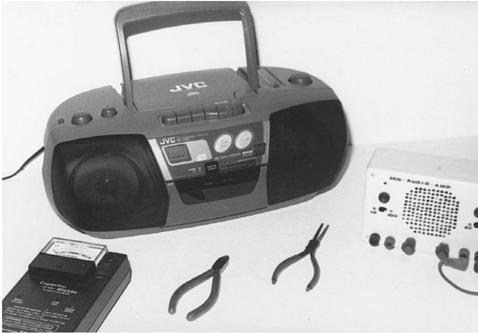
6-24 A boom-box CD player also may have an AM/FM/MPX receiver and a cassette player.
