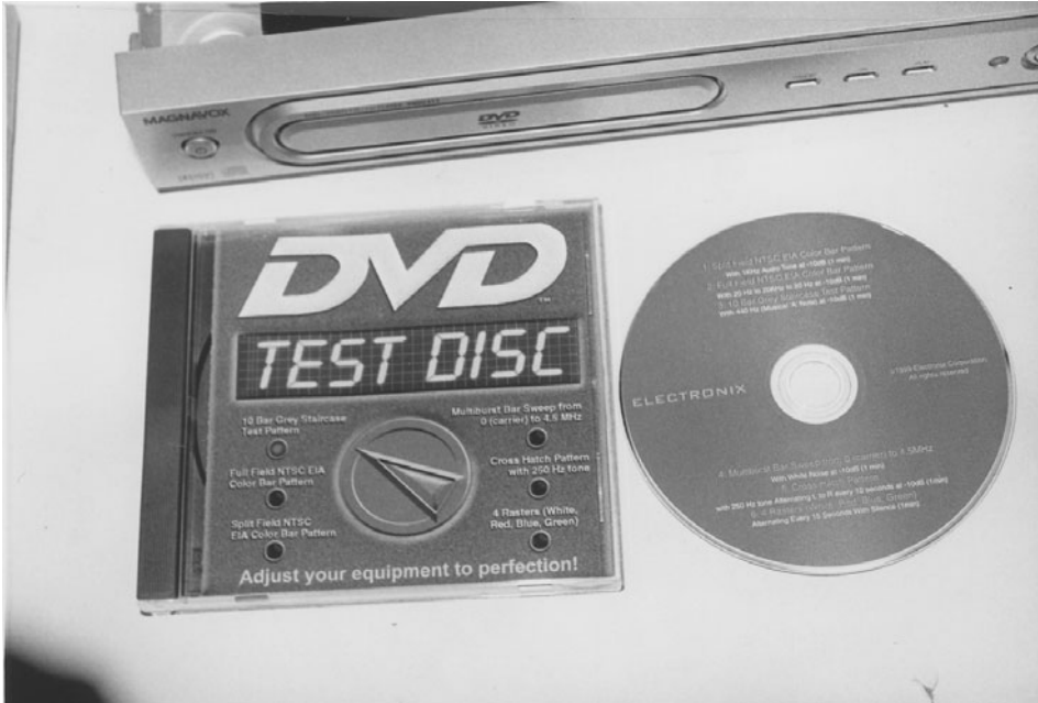
13-20 A DVD test disc can check the color-bar pattern, full-field pattern, grey-staircase test pattern, multiburst bar sweep, cross-hatch, and white, red, blue, and green rasters.
