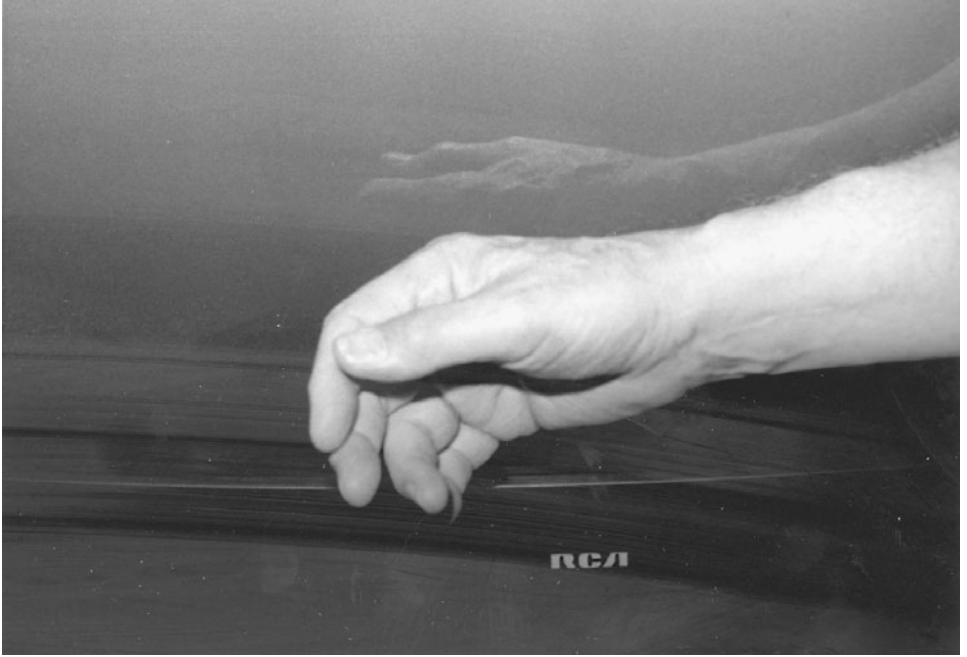
1-4 Place your arm next to the picture tube and notice if the hair rises, indicating high voltage.
