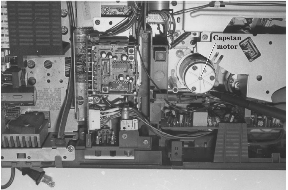
11-8 Check the capstan motor for erratic or intermittent rotation of the tape.
