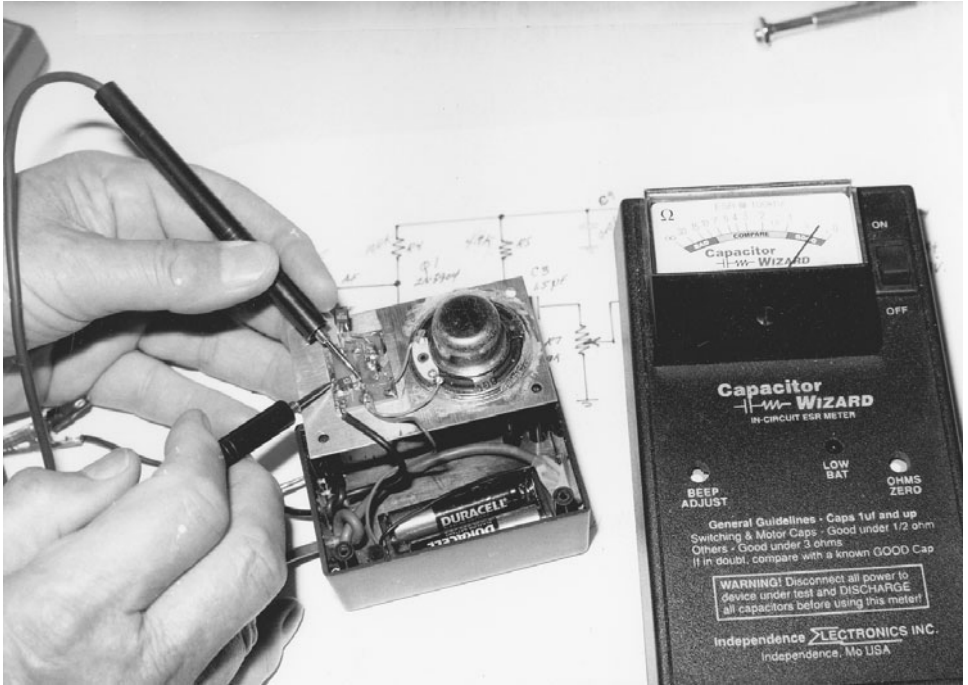
3-16 Check the electrolytic capacitors on the good scale of an ESR meter.
