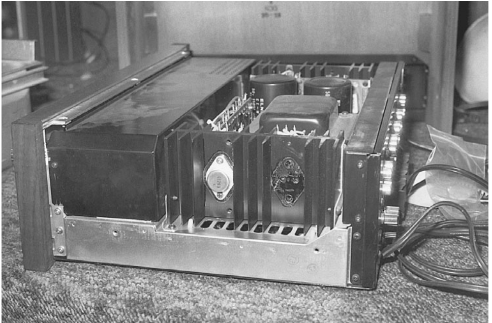
8-18 You will find several different voltage circuits with transistor and zener diode regulators within a large stereo amp receiver.
