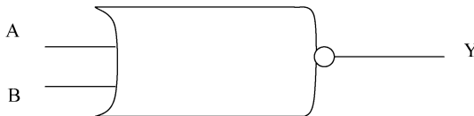
FIGURE 7.1.5 Boolean logic truth table and symbol for a NOR gate.
