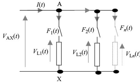
Figure 2.5 Parallel-switched inductors
