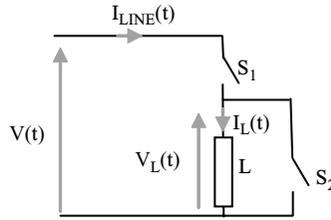
Figure 2.5(a) Single-switched inductors
