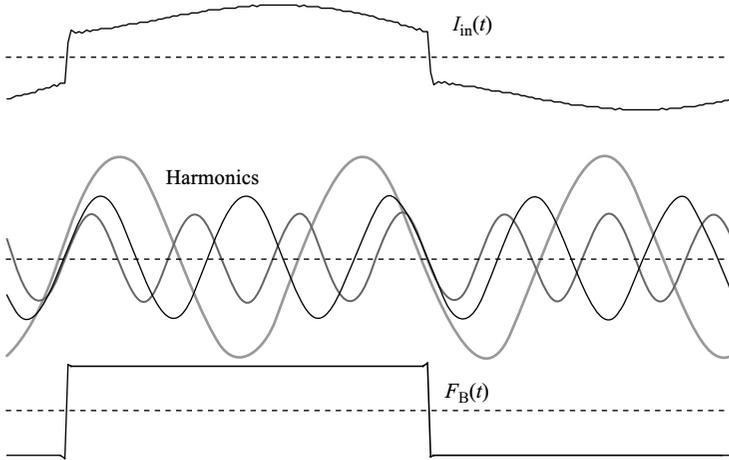
Figure 4.4 Individual line current harmonics
