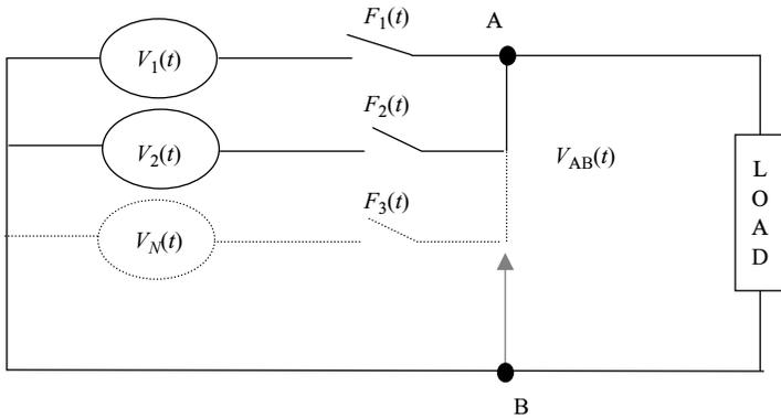
Figure 2.11 Superposition theorem
