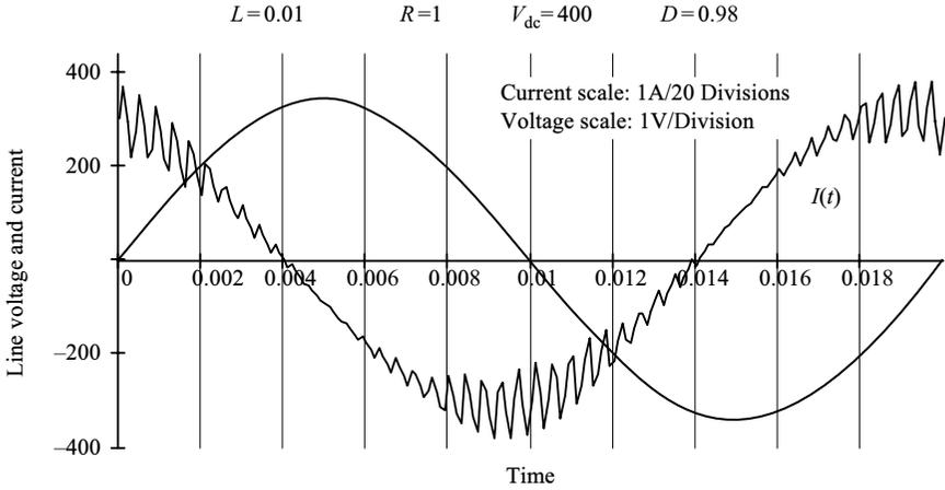
Figure 20.3 Voltage and current, leading
