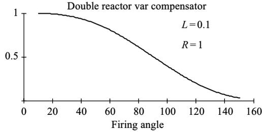
Figure 18.10 Produced inductive reactive power
