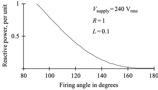
Figure 18.4 Produced inductive reactive power
