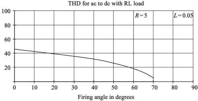
Figure 4.6 The total harmonic distortion
