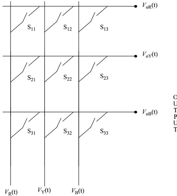
Figure 14.1 *The matrix converter*
