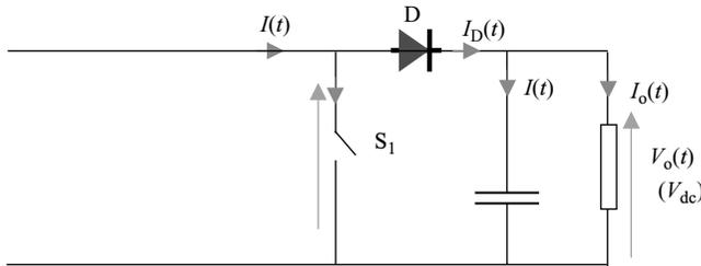
Figure 2.13 Parallel RC switched network
