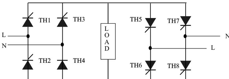
Figure 17.1 The envelope cyclo-converter
