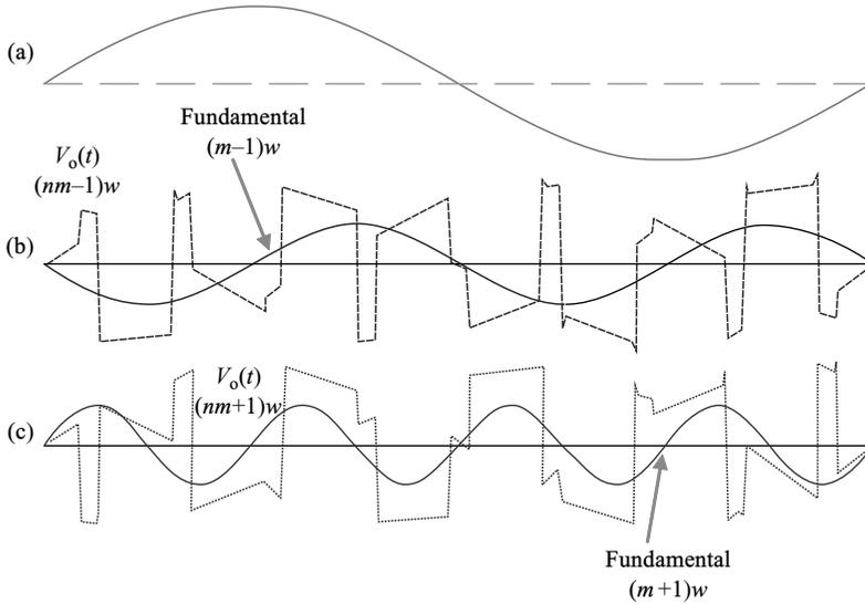
Figure 14.6 Output voltage
