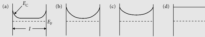
Figure 10.2. Schematic to illustrate the different regimes of band-bending within a crystal grain of dimension l . In (a) is shown the situation where N > N_t/l and the depletion width W is much less than l/2 . (b) This represents the case N = N_t/l , where the two depletion layers just meet at the centre of the grain; (c) applies to the case where N < N_t/l but where band-bending is still finite—note that the lowest point in the conduction band has moved further away from the Fermi level; (d) corresponds to low doping levels where the band-bending is now negligibly small and the conduction band lies far above the Fermi level. This last situation is characterized by the inequality \lambda_D > l , where \lambda_D is the Debye screening length.
