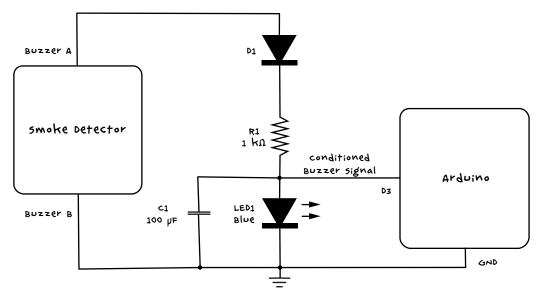
FIGURE 7-3: SCHEMATIC FOR THE FIRE ALARM
