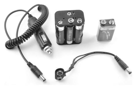
FIGURE 9-10: OPTIONS FOR POWERING THE ARDUINO
