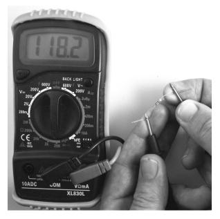
FIGURE B-13: MEASURING RESISTANCE WITH A MULTIMETER
