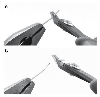
FIGURE B-1: STRIPPING WIRES
