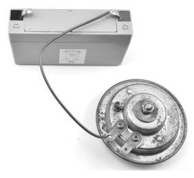
FIGURE 4-6: CONNECTING THE HORN AND BATTERY
