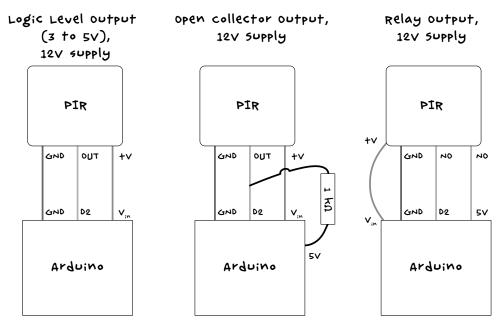
FIGURE 4-14: CONNECTING DIFFERENT TYPES OF PIR MODULE TO THE ARDUINO
