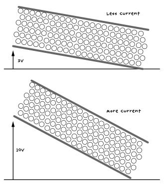
FIGURE 2-3: VOLTAGE AND CURRENT
