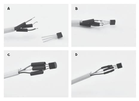
FIGURE 7-14: USING HEATSHRINK ON THE TMP36 LEAD
