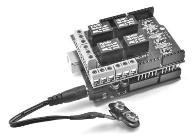
FIGURE 9-9: ATTACHING THE BATTERY LEAD TO THE ARDUINO
