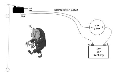
FIGURE 4-5: SCHEMATIC FOR THE TRIP WIRE ALARM
