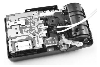
FIGURE 9-6: LEADS SOLDERED TO THE TRIGGER CONTACTS
