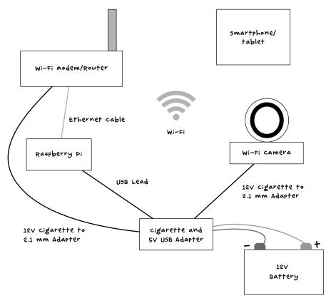
FIGURE 5-11: SCHEMATIC FOR THE WI-FI CAMERA SYSTEM
