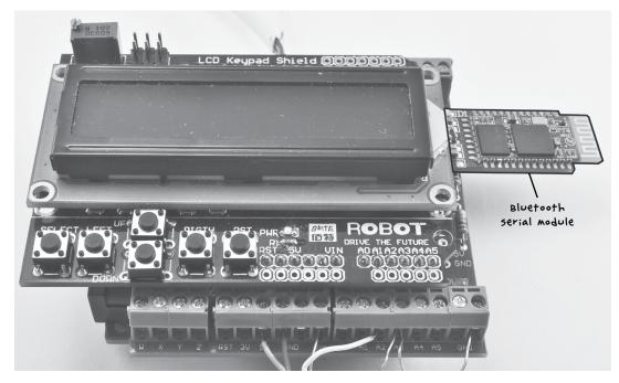
FIGURE 8-6: ADDING BLUETOOTH TO AN ARDUINO
