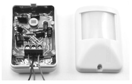
FIGURE 4-13: A PIR MODULE INTENDED FOR INTRUDER ALARMS
