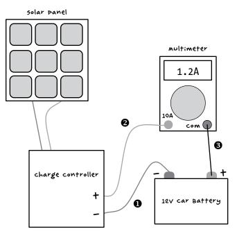
FIGURE 2-5: SOLAR PANEL WIRING DIAGRAM
