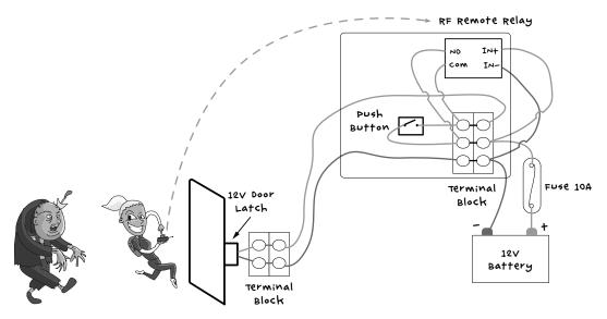
FIGURE 6-10: SCHEMATIC FOR THE ELECTRICAL DOOR LATCH WITH A WIRELESS REMOTE
