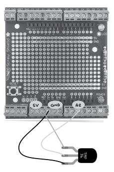
FIGURE 7–12: THE WIRING DIAGRAM FOR THE TEMPERATURE ALARM
