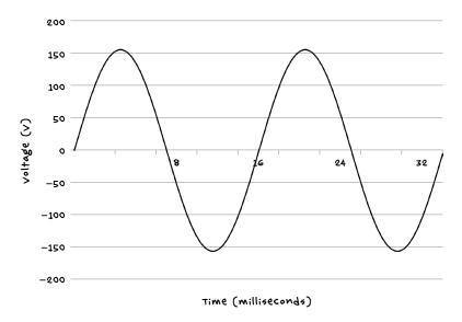
FIGURE 2-4: ALTERNATING CURRENT (AC)
