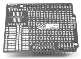
FIGURE 11-4: A PROTOSHIELD WITH HEADER PINS ATTACHED
