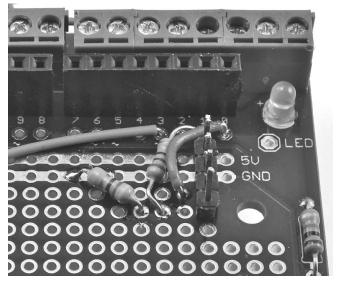
FIGURE 8-9: SOLDERING THE RESISTORS AND CONNECTING WIRE
