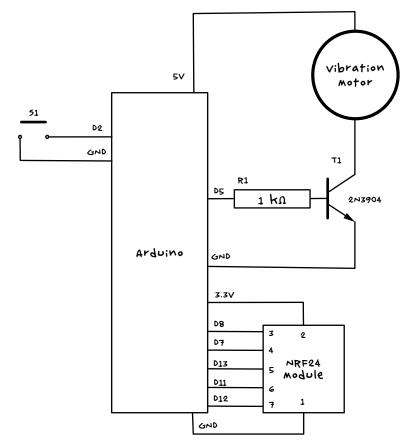
FIGURE 11-3: THE SCHEMATIC FOR ONE HAPTIC COMMUNICATOR
