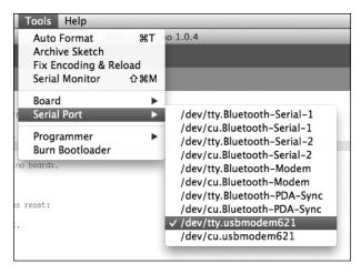
FIGURE C-3: SELECTING THE ARDUINO SERIAL PORT
