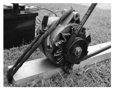
FIGURE 2-15: ATTACHING THE ALTERNATOR TO THE 2×4
