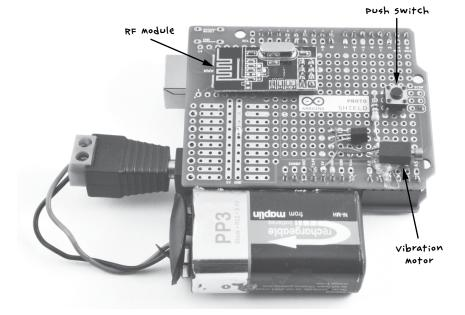
FIGURE 11-2: A HAPTIC COMMUNICATOR
