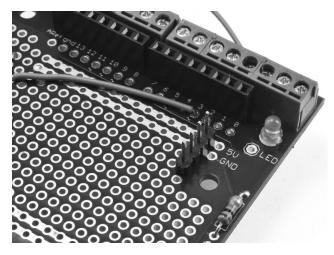
FIGURE 8-8: THE HEADER PINS SOLDERED IN PLACE
