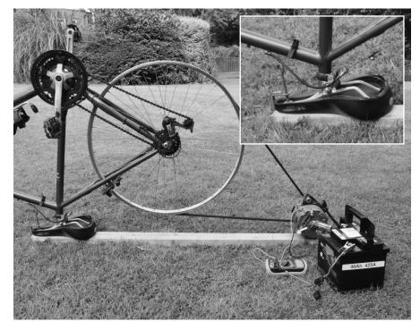
FIGURE 2-14: THE MECHANICAL ARRANGEMENT OF BIKE AND ALTERNATOR
