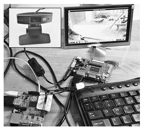
FIGURE 5-5: ZOMBIE WEBCAM AND MOVEMENT ALARM
