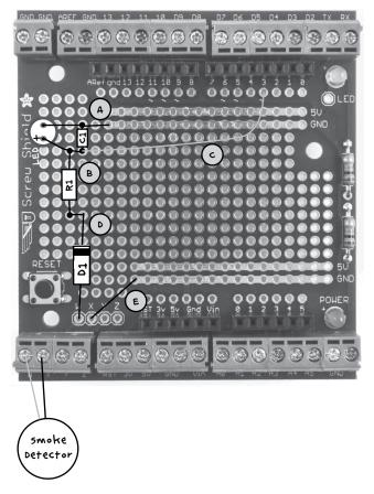
FIGURE 7-7: WIRING DIAGRAM FOR THE SCREWSHIELD
