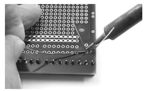
FIGURE B-G: SOLDERING A COMPONENT LEG TO A PCB
