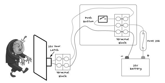
FIGURE 6-5: SCHEMATIC FOR THE ELECTRICAL DOOR LATCH
