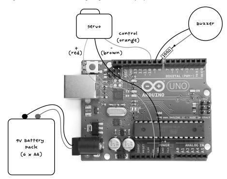
FIGURE 9-12: WIRING DIAGRAM FOR THE DISTRACTOR
