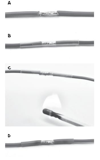
FIGURE B-8: APPLYING CLEAR HEATSHRINK TUBING OVER JOINED WIRES
