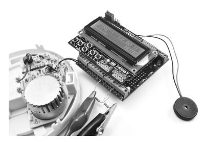
FIGURE 7-2: TESTING THE FINISHED FIRE ALARM. IN YOUR BASE, THE DETECTOR WILL BE CONNECTED TO THE ARDUINO BY A LONG LEAD.
