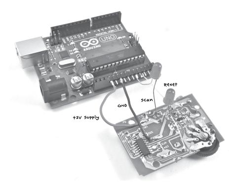
FIGURE 10-10: THE ARDUINO CONNECTED TO THE RADIO
