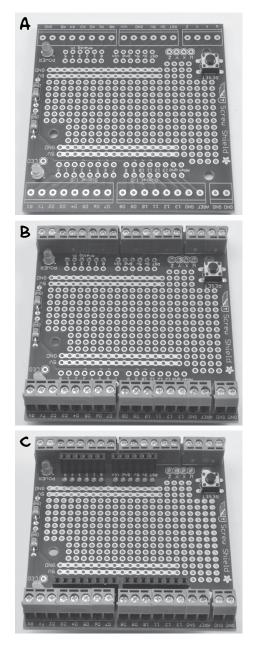
FIGURE C-8: ASSEMBLING THE SCREWSHIELD
