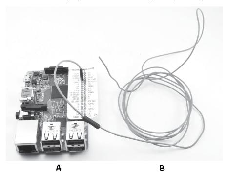
FIGURE 10-2: ATTACHING THE ANTENNA
