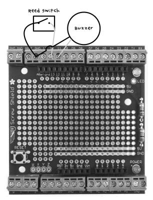
FIGURE 6-13: WIRING DIAGRAM FOR THE DOOR SENSOR
