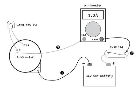
FIGURE 2-17: WIRING DIAGRAM FOR THE CYCLE CHARGER
