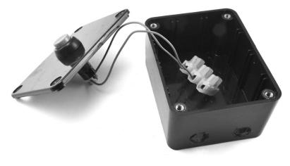
FIGURE 6-6: MAKING A SWITCH BOX. NOTE THE TWO HOLES ON THE SMALL SIDE FACING THE CAMERA, WHICH ARE FOR THE BATTERY AND LATCH WIRES.
