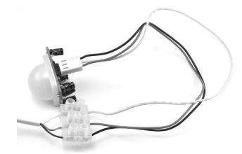
FIGURE 4-11: PIR LEAD AND TERMINAL BLOCK
