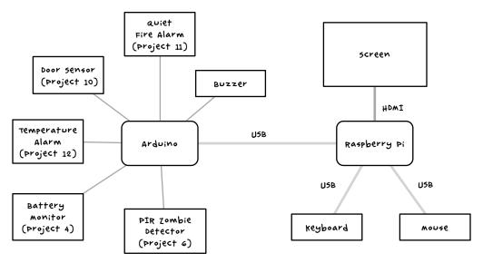
FIGURE 8-3: A SCHEMATIC OF THE CONTROL CENTER
