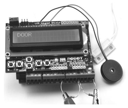
FIGURE 6-14: THE COMPLETED DOOR SENSOR
