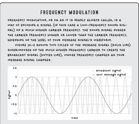
FIGURE 10-3: FREQUENCY MODULATION
