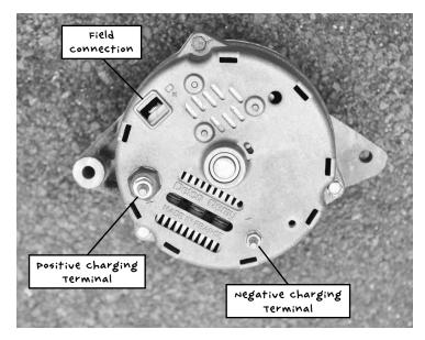
FIGURE 2-16: DELCO LRA443 ALTERNATOR (FROM THE 19805)
