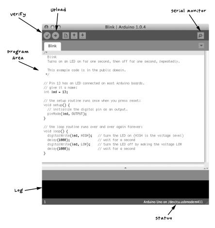
FIGURE C-2: THE ARDUINO IDE WINDOW
