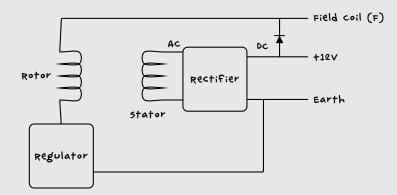
FIGURE 2-13: THE SCHEMATIC DIAGRAM FOR AN AUTOMOTIVE ALTERNATOR
