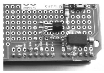
FIGURE 11-9: ATTACHING THE VIBRATION MOTOR
