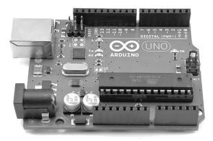
FIGURE 1-5: AN ARDUINO MICROCONTROLLER BOARD
