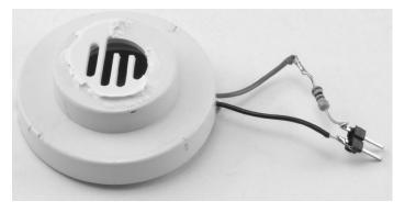
FIGURE 9-14: SOLDERING THE BUZZER, RESISTOR, AND HEADER PINS
