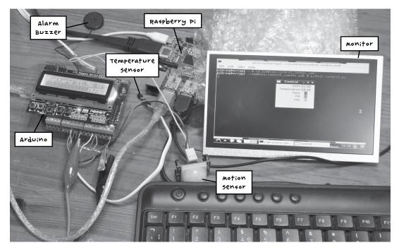
FIGURE 8-2: RASPBERRY PI AND ARDUINO WORKING TOGETHER
