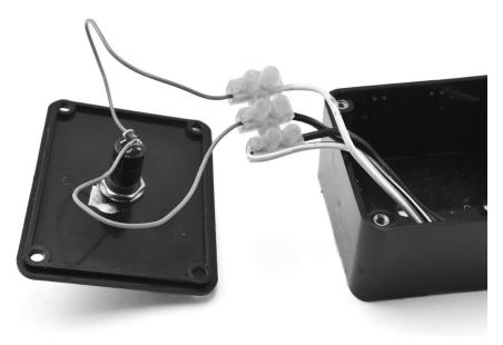
FIGURE 6-9: WIRING UP THE SWITCH BOX
