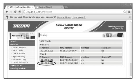
FIGURE 5-13: FINDING THE IP ADDRESS OF THE CAMERA
