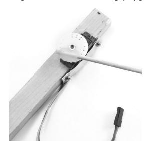
FIGURE 9-18: ATTACHING THE FLAG TO THE SERVO
