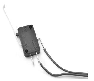
FIGURE 4-7: SOLDERING WIRES TO THE SWITCH
