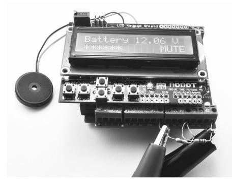
FIGURE 3-8: BATTERY MONITOR
