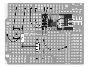
FIGURE 11-7: WIRING DIAGRAM FROM THE UNDERSIDE OF THE PROTOSHIELD
