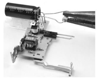
FIGURE 9-5: DISCHARGING THE CAPACITOR
