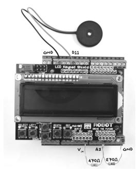
FIGURE 3-11: CONNECTING COMPONENTS TO THE SCREWSHIELD
