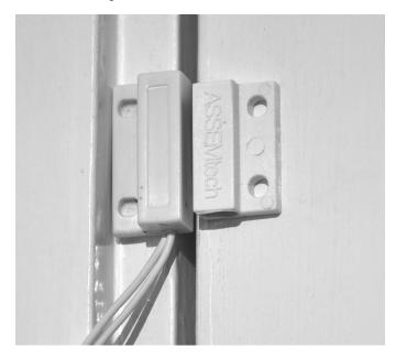
FIGURE 6-15: REED SWITCH AND MAGNET ON A DOOR
