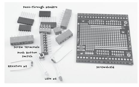
FIGURE C-7: THE PARTS OF ADAFRUIT'S PROTO-SCREWSHIELD
