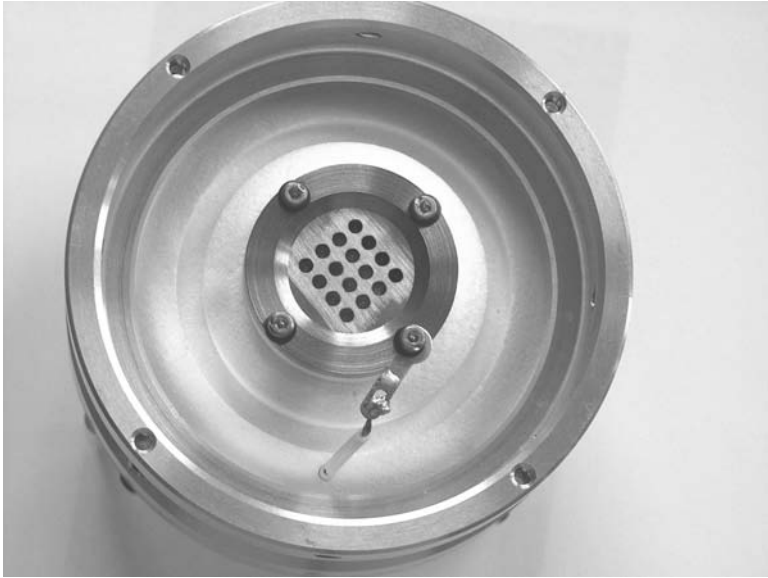
FIGURE 11.9 FEEP multi-emitter design. (Source: Austrian Research Centre.)
