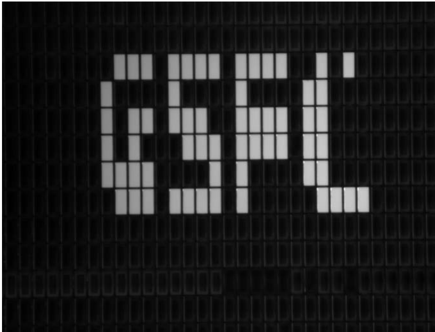
FIGURE 7.9 Optical transmission image of a pattern written with the microshutter array ( Source: NASA GSFC. )
