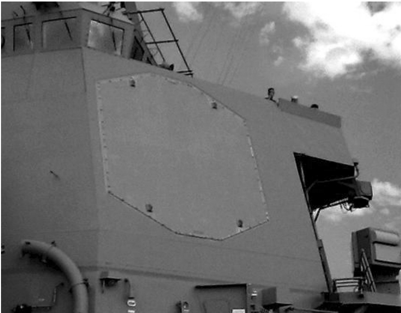
FIGURE 8.8 Photograph of a SPY-1 radar array, which is an example of a electrically steered antenna that relies on an array of smaller antennas combined with phase shifters. (Photo by F.H. Sanders. Courtesy of the Institute for Telecommunication Sciences.)
