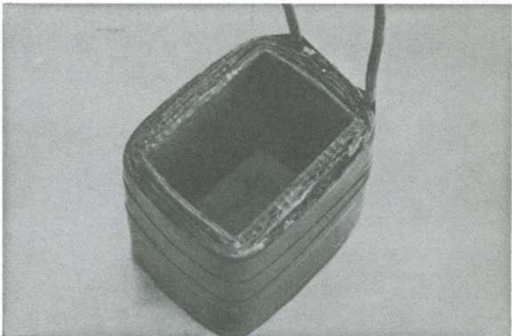
Fig. 10-30. The winding form taped and ready for rewinding. All of the windings except the primary have been stripped away.
