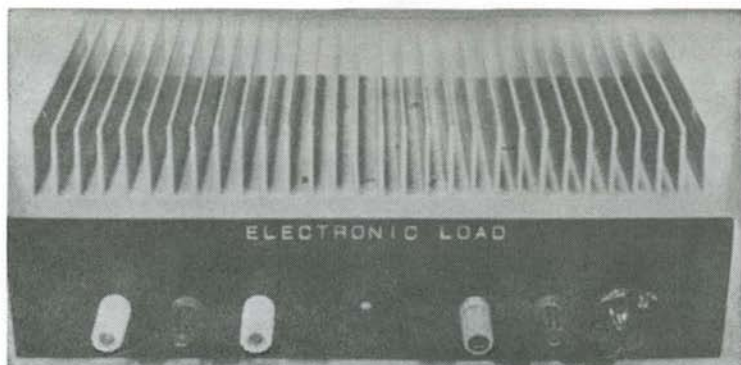
Fig. 1-67. The Power Waster. This electronic load is adjustable from 0 to 10 A and can dissipate up to 300 watts. The unit is built upon a piece of heat-sink extrusion and has both reverse polarity and thermal overload protection.
