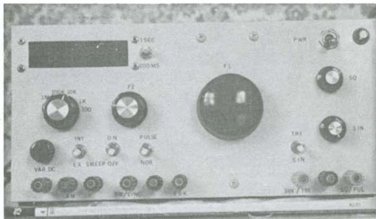
Fig. 3-25. The completed swept function generator. The knob labeled F1 is the primary frequency control and is mounted on a 3:1 gear drive. The SIN/TRI output jack also provides a ramp function. All unlabeled jacks are grounds, except the jack, far left, which is the variable dc output.
