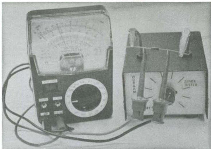
Fig. 2-31. Unit with a zener diode being tested and showing proper hookup to the VOM. Note that the VOM is indicating 8.6 volts even though the tester voltage output is 28 volts. Don't forget to set the VOM to measure dc voltage. It doesn't show up very well in the photo, but I used red wire for the plus alligator clip and black for the negative. These wires were then inserted into 2 phone tip jacks on the top of the case.
