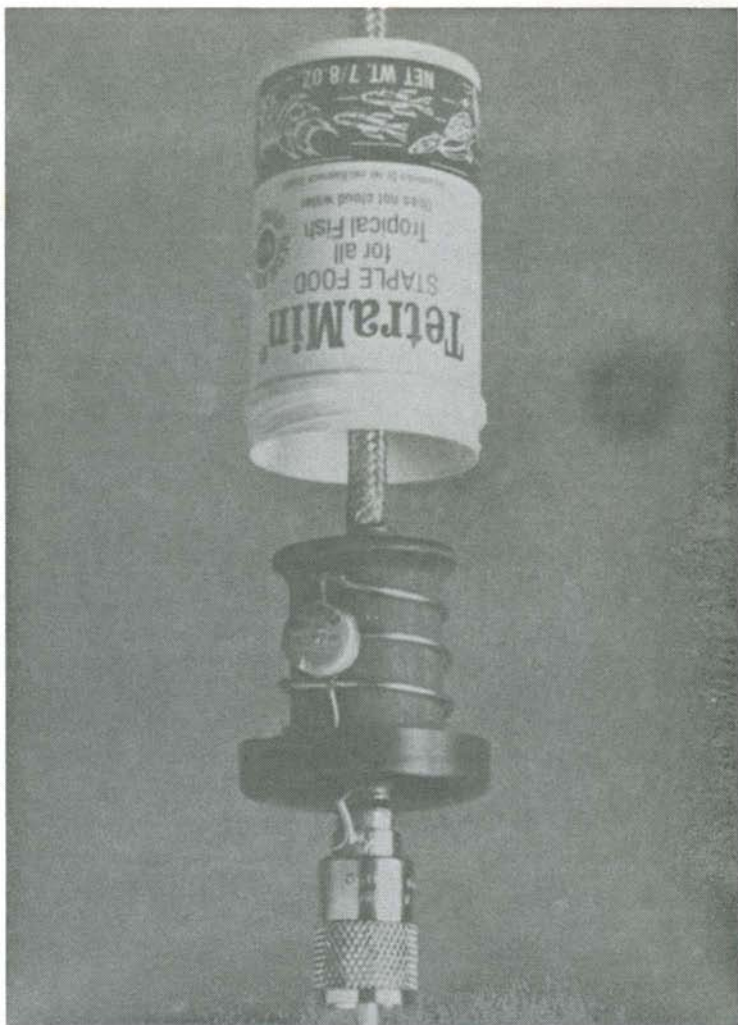
Fig. 7-28. The coil protective cover has been removed in this picture to show details of the base coil.
