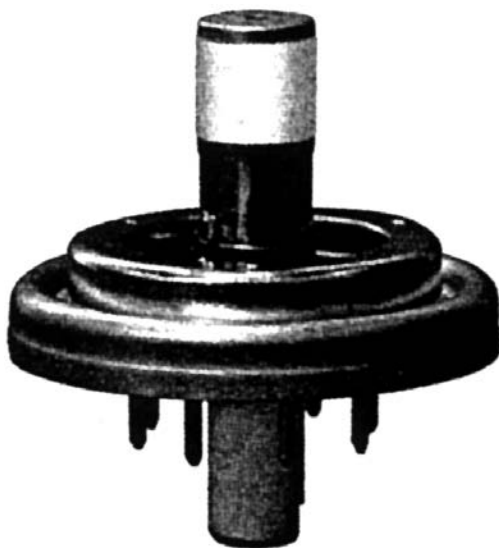
FIGURE 5.22 Photograph of a typical oxide cathode. (Source: Varian/Eimac.)
