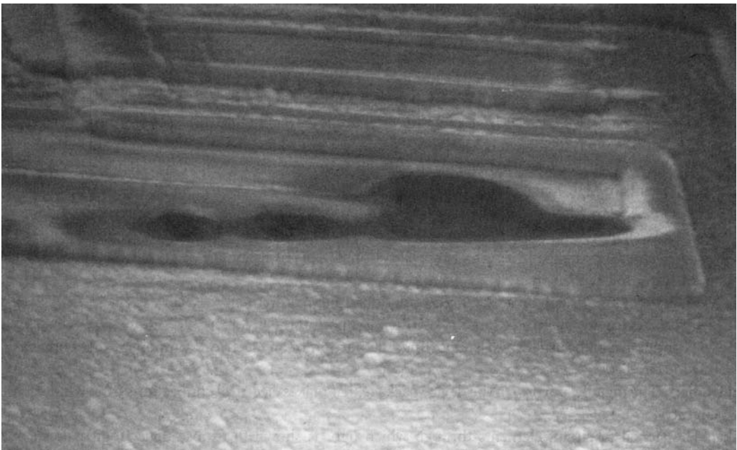
FIGURE 7.162 Passivation fault extending under the metallization.
