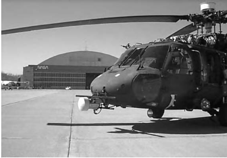
FIGURE 20.11 Honeywell 35 GHz biphas modulated CW obstacle avoidance radar ( http://ccf.arc.nasa.gov/dx/basket/pix/RASCAL.jpg ). (Photo: Dominic Hart.)
