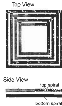
FIGURE 4.32. Stacked transformer with completely overlapping spirals.
