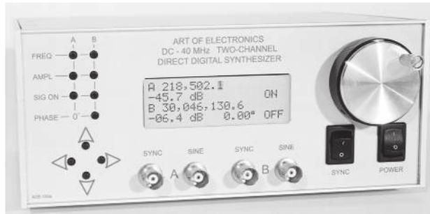
**Figure 15.6.** Dual DDS frequency synthesizer of Figure 15.5, with panel controls (eleven buttons and one rotary encoder dial) and readout. (Designed, built, coded, and documented with excellence by Jonathan Wolff; see [www.artofelectronics.com/synthesizer](http://www.artofelectronics.com/synthesizer))
