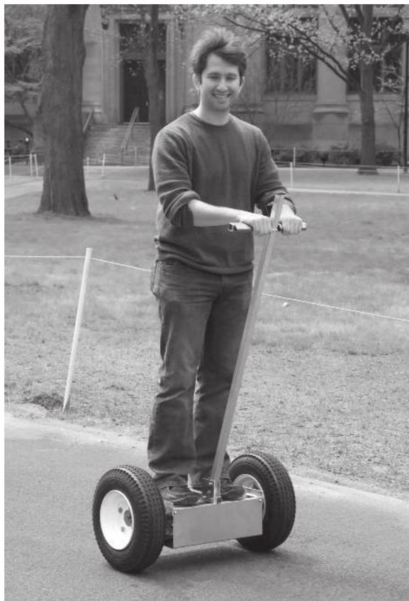
**Figure 15.17.** Stabilized two-wheel contraption, demonstrated by its creator (Jesse Colman-McGill).
