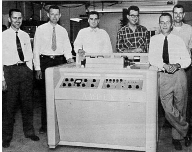
**Figure 10.2** The Ampex team and the first professional videotape recorder.
