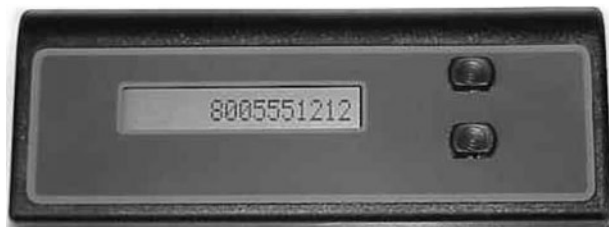
Figure 28-1 DTMF decoder display
