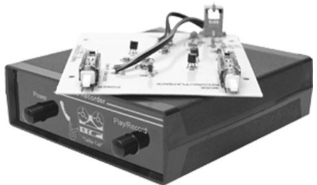
Figure 9-1 Automatic telephone recording switch
