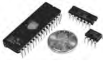
Figure 2-7 Examples of integrated circuits. These are “dual in-line” (DIP) styles.
