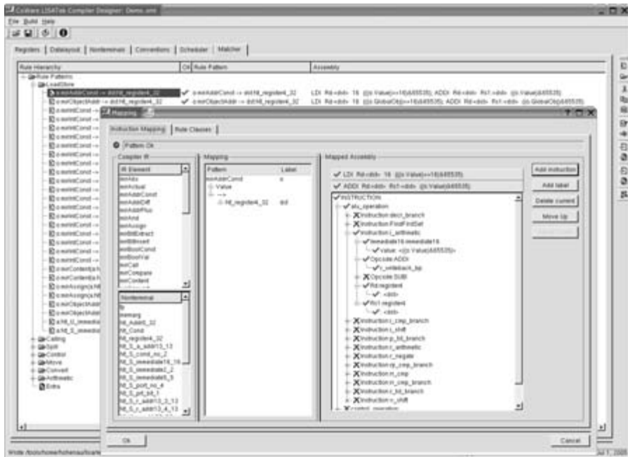
Figure 8.26 GUI for interactive compiler retargeting (code selector view)
