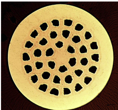
Figure 2.18 A typical commercial 36 multifilament \text{MgB}_2 round \sim 1 mm diameter wire with 60- \mu\text{m} filaments, fabricated using the powder-in-tube method. Courtesy of M. Tomisc, HyperTech, Columbus, OH.
