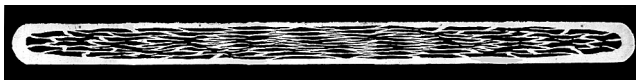
Figure 2.21 Typical multifilamentary BSCCO-2223 PIT tapes (dimension 0.3\text{mm} \times 4\text{mm} ). Courtesy of Sumitomo Electric Industries, Ltd.
