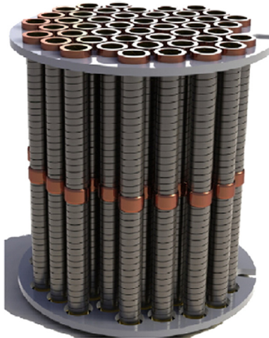
Figure 9.14 A module of Bi-2212 elements (Nexans picture) (Tixador, 2010). © 2010
