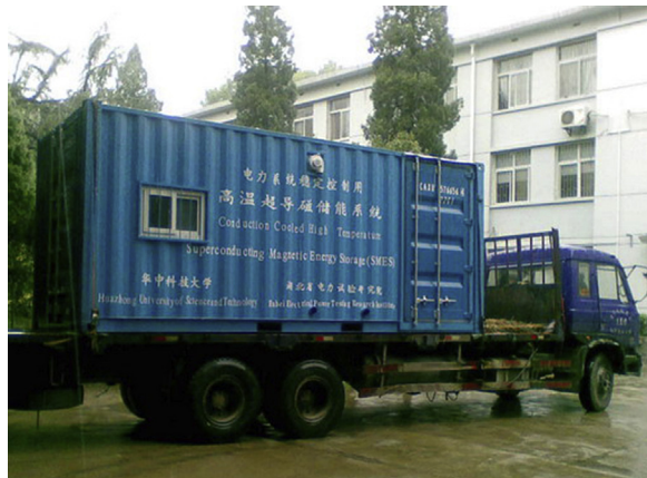
Figure 13.19 Assembled 35 kJ/7 kVA high-temperature superconducting magnetic energy storage for field test.
